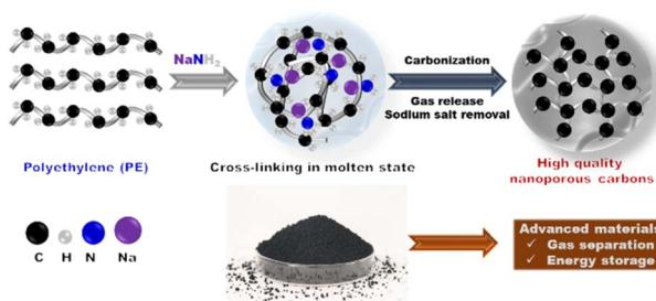
**A tandem approach for waste-to-nanomaterial transformation towards polyethylene recycling**
