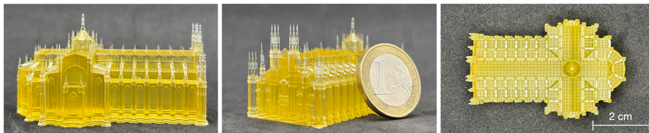
Fig. 3 3D printing performances of MEIA-based resins. High-resolution 3D-printed reproduction of Milan's Dome printed using 40 mol% of Ile-MEIA. Object size is 39 × 60 × 33 mm, spiers are as thin as 0.5 mm.
