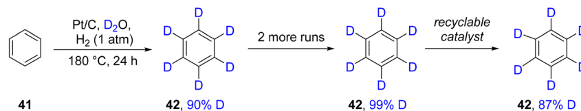
Scheme 13 Deuteration of benzene using Pt/C/D 2 O according to Sadjadi et al. 94
