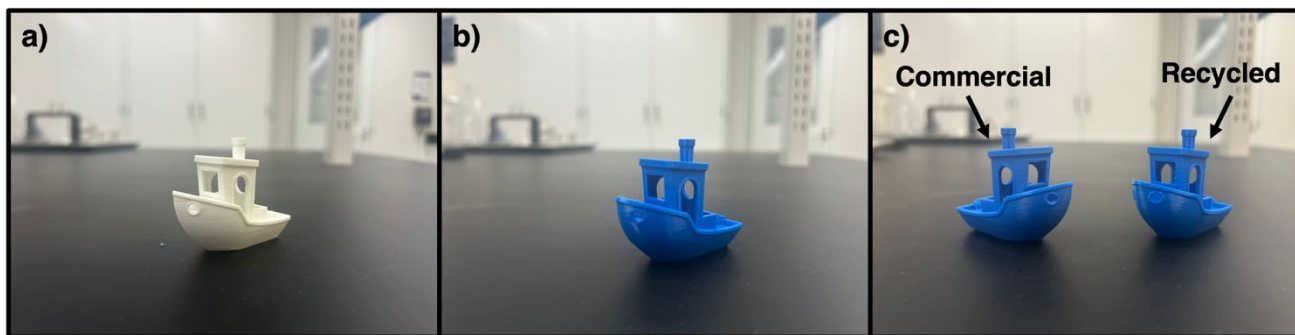
Figure 7. 3D printed 3DBenchys of 6.0 cm length, 3.1 cm width and 4.8 cm height from a) recycled white filament and b) recycled blue filament. c) Comparison of commercial and recycled filaments on a final 3D printed object.
