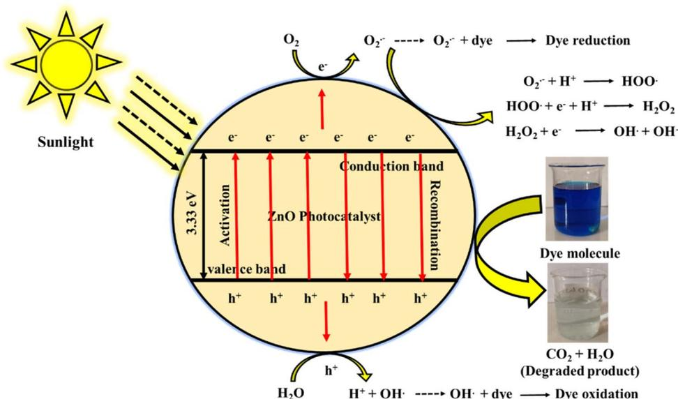
Fig. 9 Mechanistic pathway for the ZnO nanoparticle-assisted photo-degradation of MB dye.
