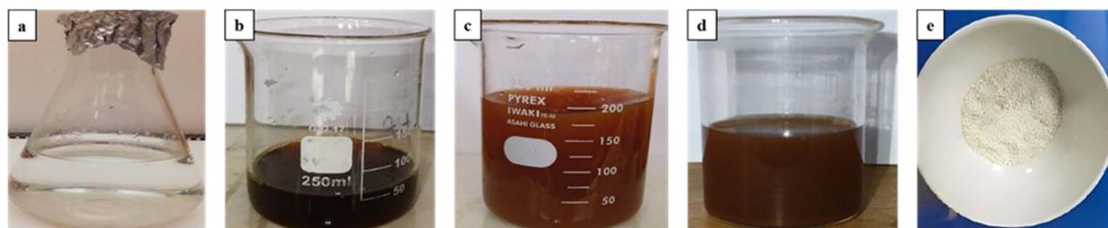
Fig. 2 Images of (a) zinc nitrate hexahydrate precursor, (b) leaf extract, and sample (c) before and (d) after microwave radiation, and (e) white ZnO nanoparticles.
