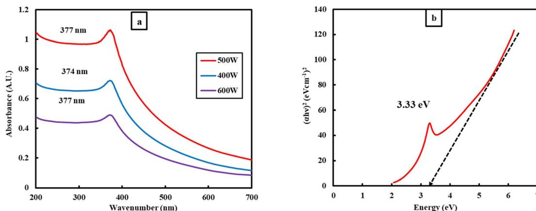
Fig. 5 (a) UV-visible spectra of the 400 W, 500 W and 600 W samples. (b) Tauc plot of ZnO nanoparticles.
