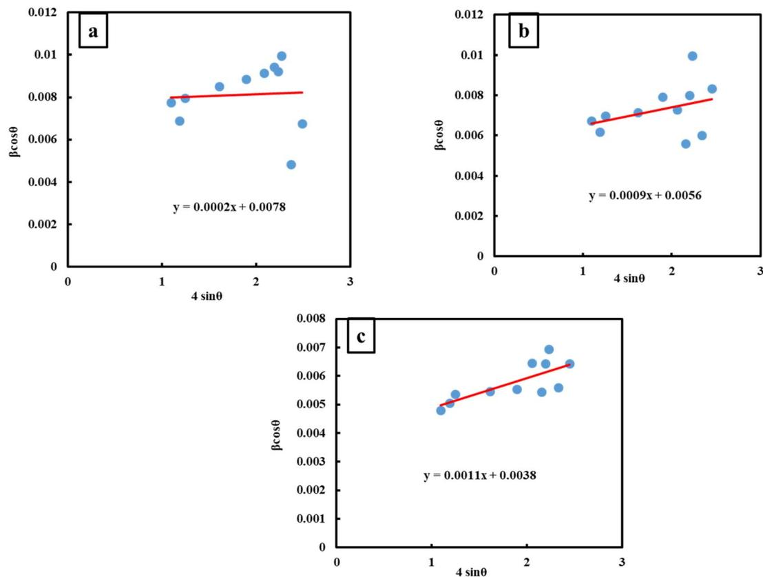
Fig. 4 W–H scheme for ZnO nanoparticles at (a) 400 W, (b) 500 W, and (c) 600 W.
