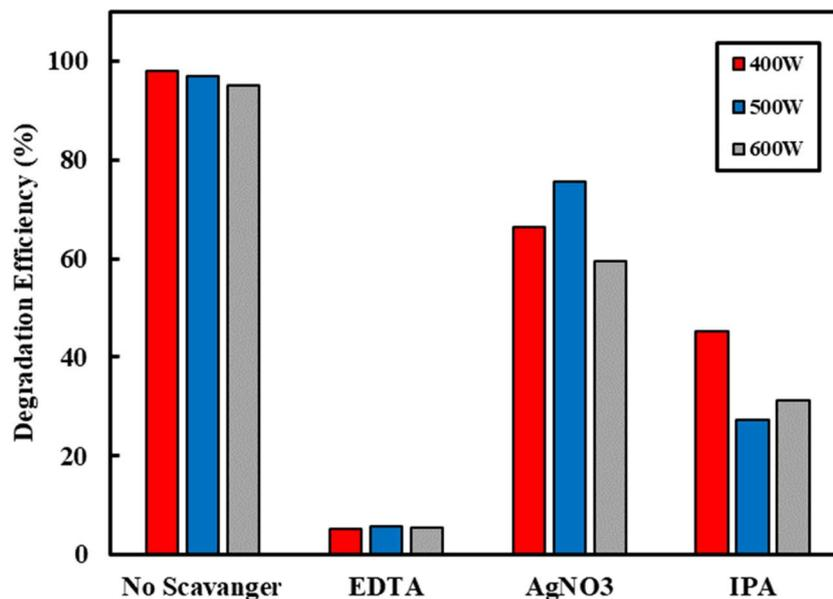
Fig. 12 Radical scavenger tests of the three synthesized ZnO nanoparticle samples prepared at 400 W, 500 W, and 600 W.
