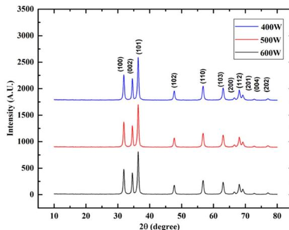
Fig. 3 XRD patterns of 400 W, 500 W and 600 W ZnO nanoparticles.
