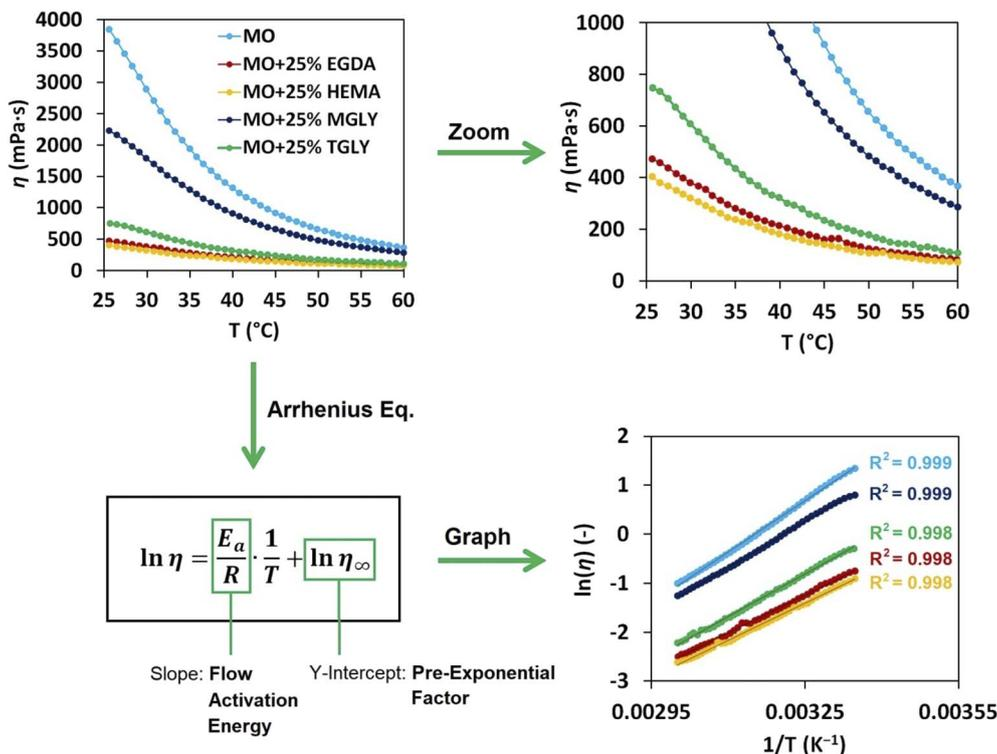
Fig. 6 The rheological investigation of diluted methacrylate vegetable oil (MO) systems containing 25 wt% of the reactive diluent used (top left) and a zoom-in (top right). The graphical interpretation of the Arrhenius equation (bottom left) applied to the investigated systems (bottom right).
