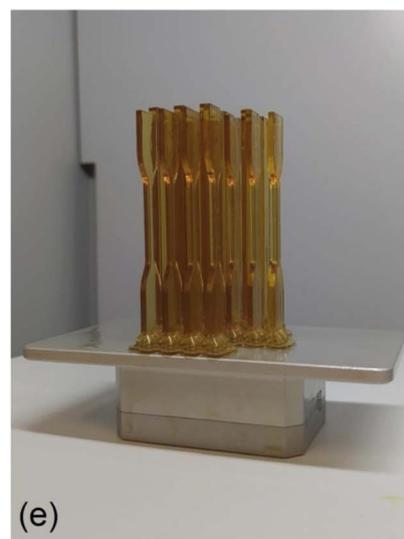
Fig. 8 The results of the mechanical tests. (a) Tensile moduli, (b) tensile strengths, (c) flexural moduli, (d) flexural strengths, and (e) the image of the 3D printed testing specimens.
