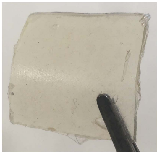
Fig. 1 Image of the material produced by curing a mixture of the HBPE with 8 equivalents of phenyldiboronic acid at 120 °C under vacuum overnight.
