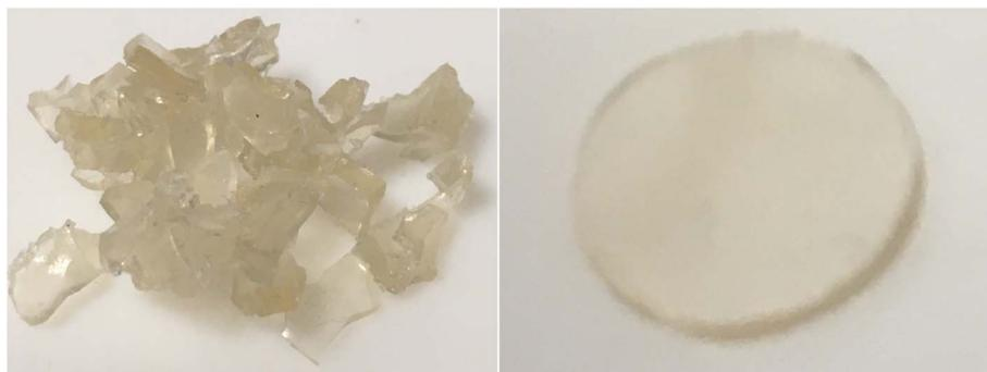
Fig. 11 Pictures of the cut pristine (left) and recast (at 120 °C) (right) dihydroxylated methyl erucate-based cross-linked HBPEs with 8 eq. of phenyl diboronic acid used as the cross-linker.
