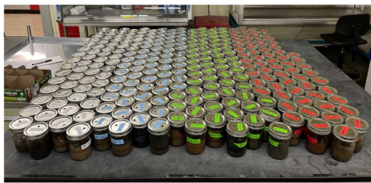
Fig. 4 120 day soil incubation featuring 264 mason jars, 22 soils, and 4 amendment groups. The incubation durations tested were 0, 1, 7, 30, and 120 days. Soils were weighed every 7–10 days, and water was added to maintain the soil saturation throughout the incubation.
