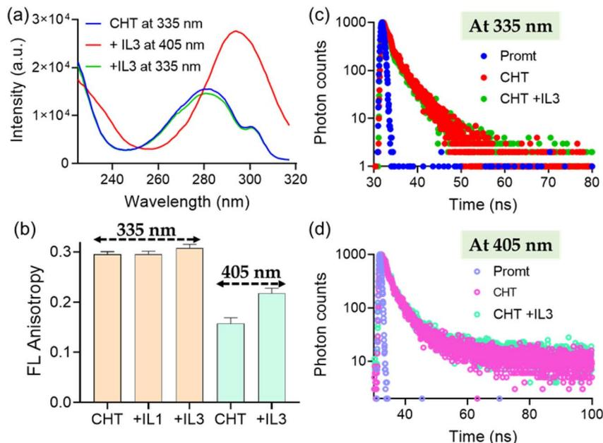
Fig. 6 (a) Fluorescence excitation spectra of CHT (0.1 mg mL<sup>-1</sup>) with IL3 (220 μM) at 335 nm and 405 nm at pH 6.5 in buffered medium. (b) Fluorescence anisotropy of CHT (0.1 mg mL<sup>-1</sup>) with IL1 and IL3 (220 μM) at 335 and 405 nm in buffered medium (at pH 6.5). Fluorescence decay spectra of CHT (0.1 mg mL<sup>-1</sup>, λ<sub>ex</sub> = 280 nm) upon addition of IL3 (220 μM) at (c) 335 and (d) 405 nm in buffered medium (at pH 6.5).
