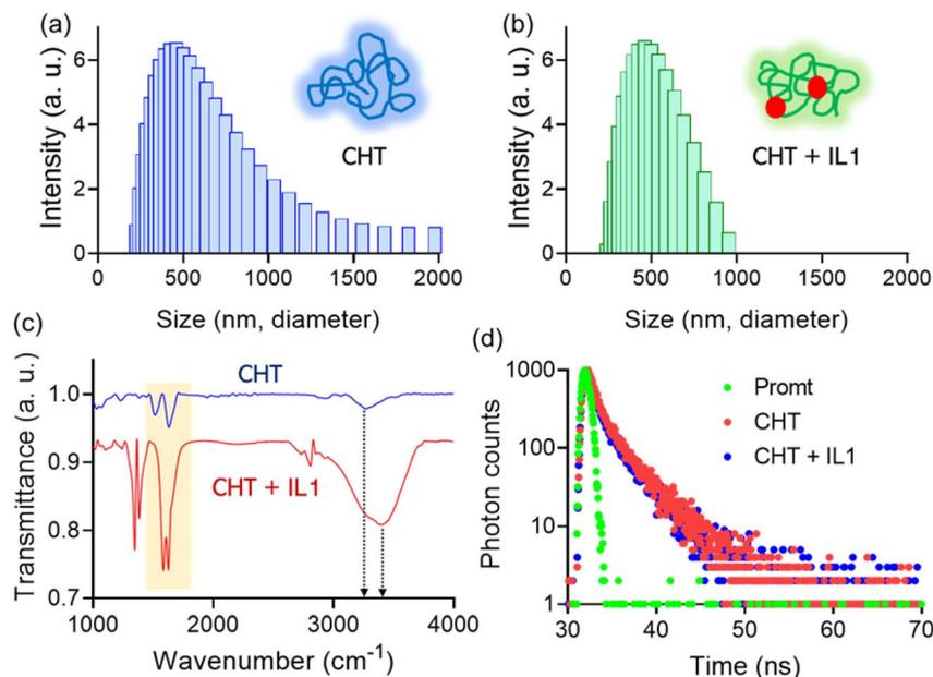
Fig. 5 Determination of the hydrodynamic diameter of CHT ( $0.1 \text{ mg mL}^{-1}$ ,  $\lambda_{\text{ex}} = 280 \text{ nm}$ ) in the (a) absence and (b) presence of IL1 ( $220 \mu\text{M}$ ) at pH 6.5 in buffered medium using DLS. (c) FT-IR spectra of CHT ( $0.1 \text{ mg mL}^{-1}$ ) with and without IL1. (d) Fluorescence decay spectra of CHT ( $0.1 \text{ mg mL}^{-1}$ ,  $\lambda_{\text{ex}} = 280 \text{ nm}$ ) at 335 nm upon addition of IL1 ( $220 \mu\text{M}$ ) at pH 6.5 in buffered medium.
