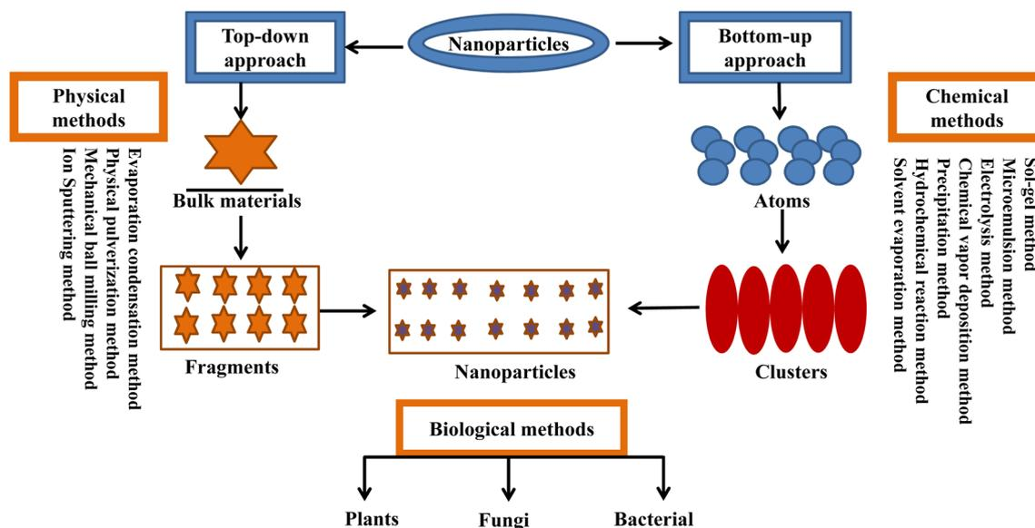
Fig. 2 Classification of synthesis methods for silica nanoparticles.
