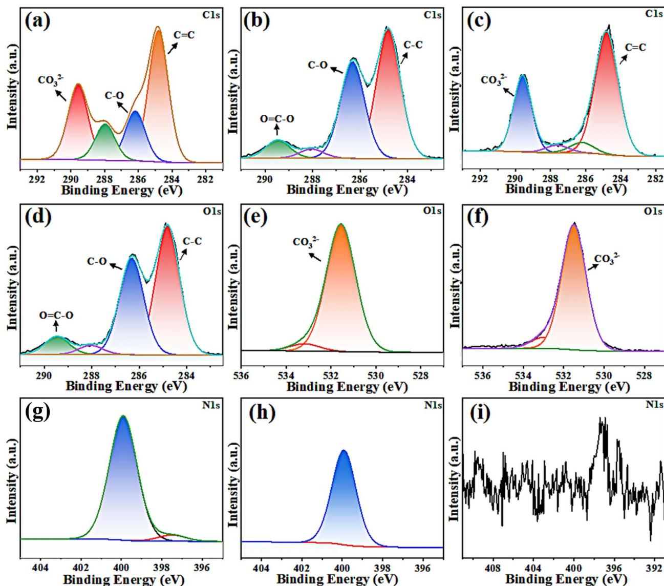
Fig. 4 High-resolution (a–c) C1s, (d–f) O1s, and (g–i) N1s spectra of ES, PEG@ES, and C-PEG@ES.
