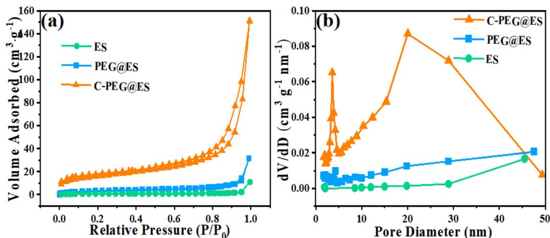
Fig. 5 (a) Nitrogen adsorption–desorption isotherms, (b) distribution curves.
