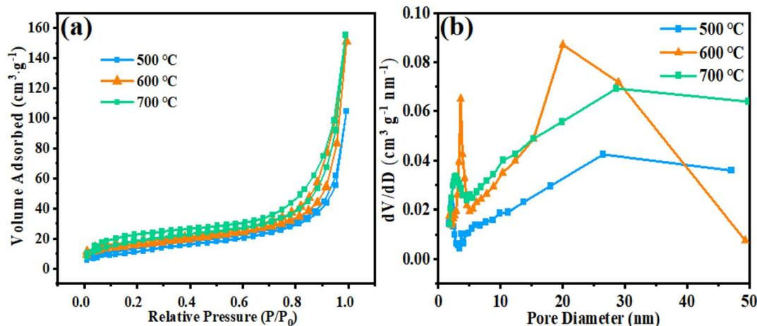
Fig. 1 (a) Nitrogen adsorption–desorption isotherms, (b) distribution curves.
