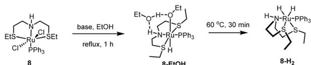
Fig. 6 Conversion of complex **8** to facial dihydride complex **8-H<sub>2</sub>**.
