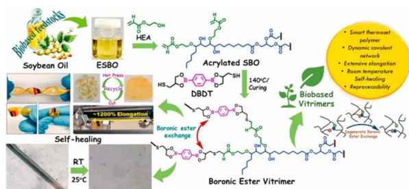
Fig. 13 Schematic of the synthesis and research of the ESBO–HEA–DBDT biobased trimer. Reproduced with permission. 72 Copyright 2025, Elsevier.
