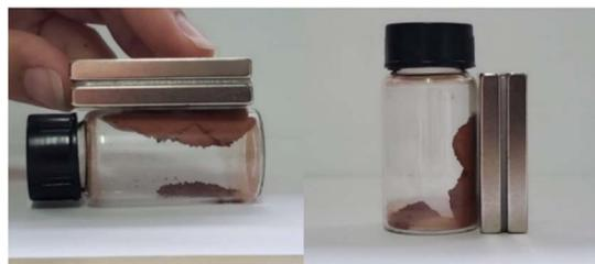
Fig. 5 Interaction of MgFe700 sample with neodymium magnet.
