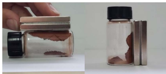
Fig. 5 Interaction of MgFe700 sample with neodymium magnet.
