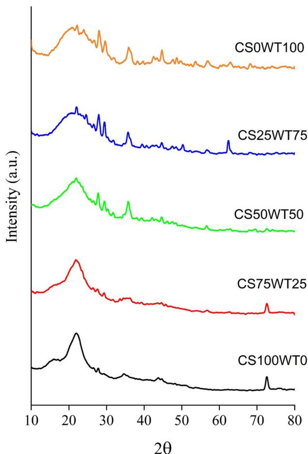
Fig. 7 XRD test results for each specimen.
