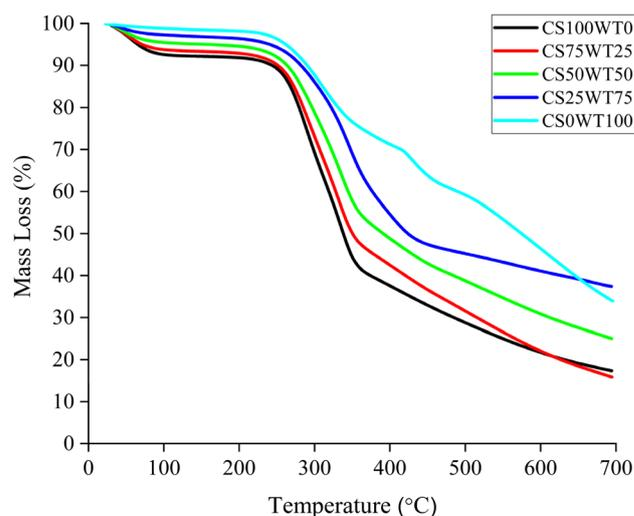
Fig. 3 TGA test results for each specimen.
