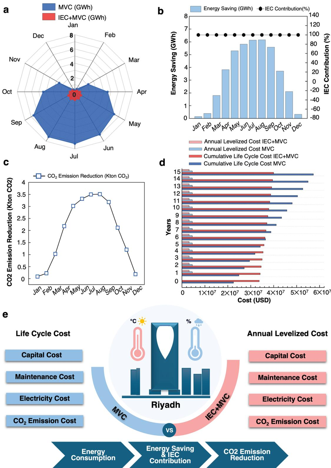
Fig. 2 (a) Comparison of energy consumption for the MVC and IEC + MVC systems in Riyadh. (b) Energy saving of the IEC + MVC system compared to the MVC system and IEC contribution in Riyadh. (c) CO<sub>2</sub> emission reduction of the IEC + MVC system compared to the MVC system in Riyadh. (d) Cost of the MVC system and IEC + MVC system in Riyadh. (e) Concept of cost analysis of MVC and IEC + MVC.
