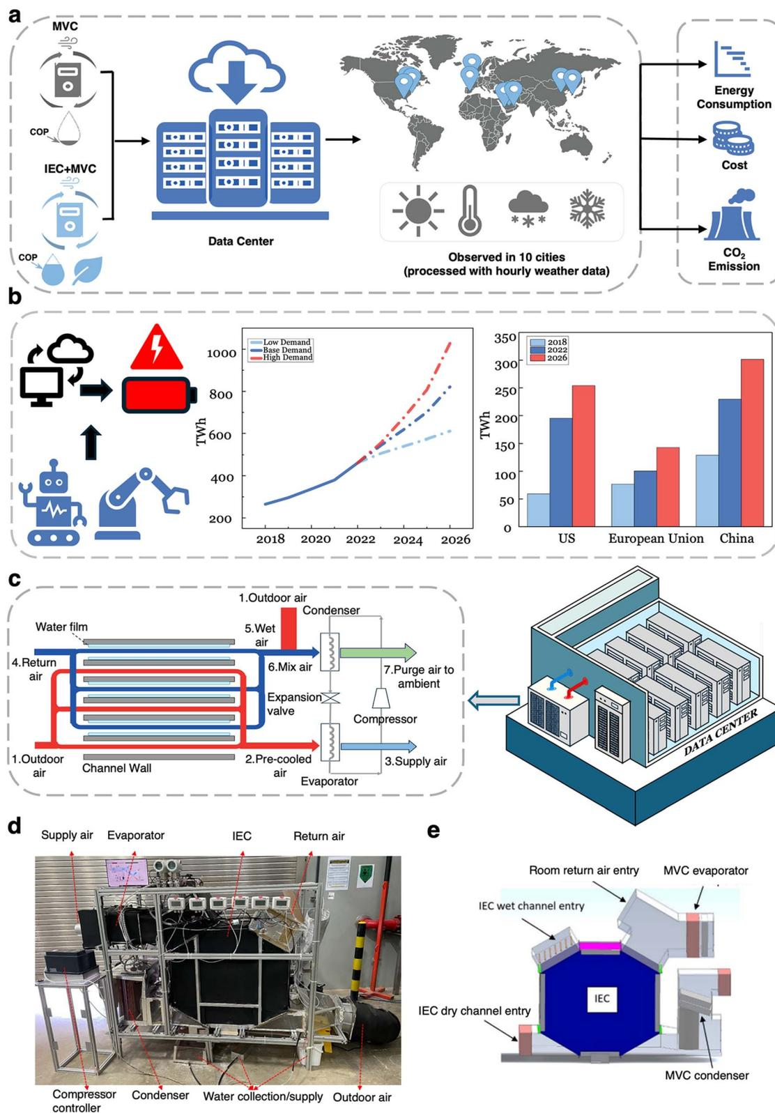
Fig. 1 (a) Research path. (b) Estimated global data centres electricity consumption from 2018 to 2026.<sup>1</sup> (c) Schematic of hybrid IEC + MVC system in a data centre.<sup>13,28–30</sup> (d) and (e) Hybrid MVC + IEC pilot at KAUST.<sup>31</sup>
