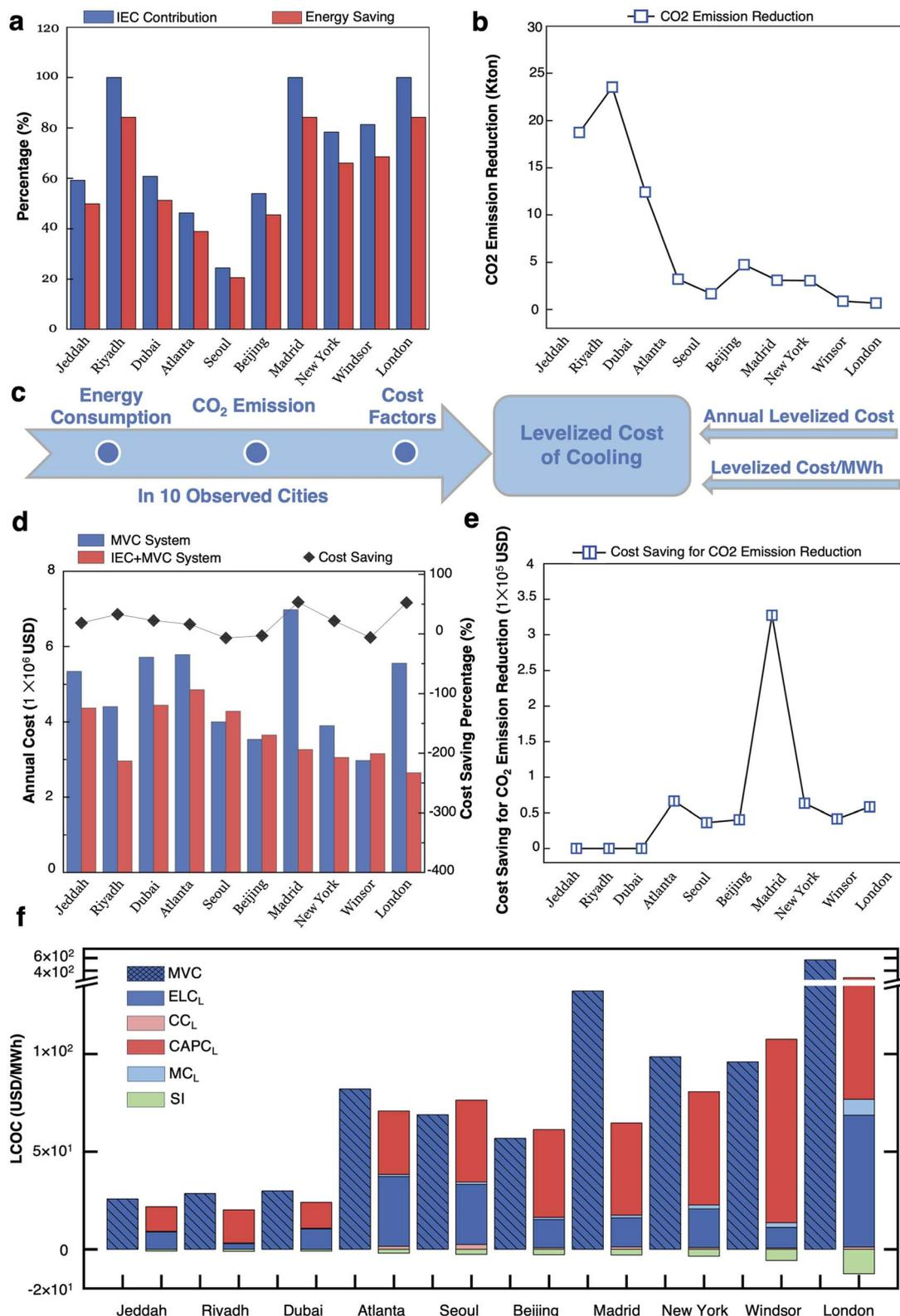
Fig. 4 (a) Annual energy saving and IEC contribution percentage in different cities. (b) CO<sub>2</sub> emission reduction for each city. (c) Concept of the levelized cost of cooling. (d) Annual levelized cost and cost saving percentage of cooling systems for each city. (e) Cost saving for CO<sub>2</sub> emission reduction for each city. (f) Comparison of LCOE (USD per MWh) for MVC and IEC + MVC systems in 10 observed cities, with distribution of cost for the hybrid IEC + MVC system.
