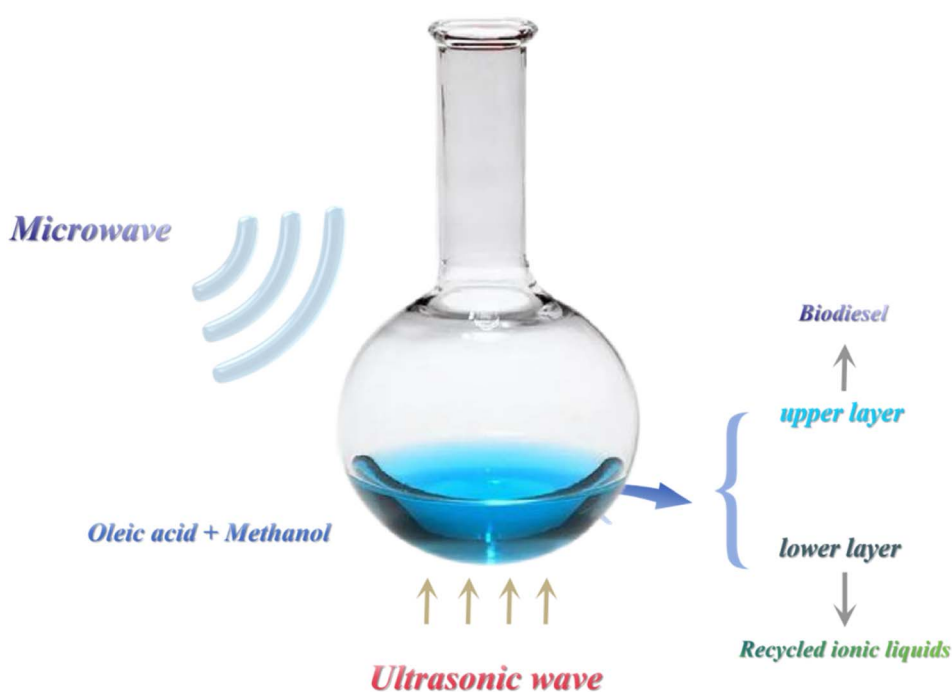
Fig. 5 Enhancement mass transfer process of ionic liquids by microwave. [Adapted from ref. 61 with permission from American Chemical Society, copyright 2024].
