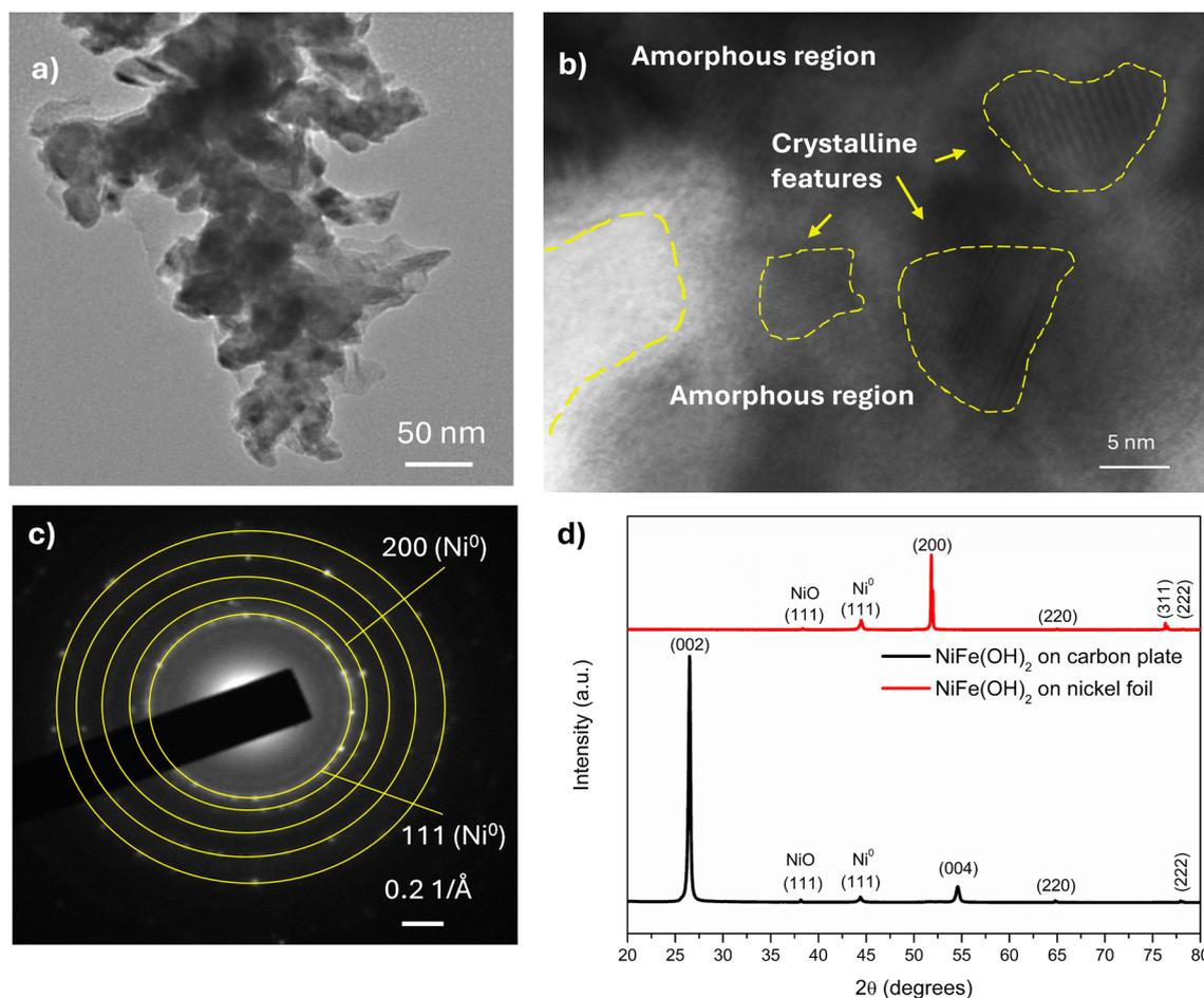
Fig. 2 (a) Low-magnification TEM image of  $\text{NiFe}(\text{OH})_2$  (b) high-resolution TEM image of  $\text{NiFe}(\text{OH})_2$  (c) SAED ring diffraction pattern of  $\text{NiFe}(\text{OH})_2$  with the relevant Miller indices of the two most prominent peaks (d) X-ray diffraction (XRD) patterns for  $\text{NiFe}(\text{OH})_2$  on a carbon plate substrate and on a Ni foil substrate.
