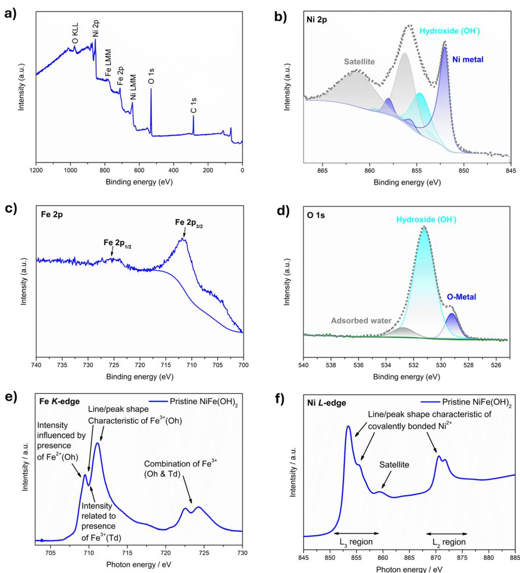
Fig. 3 (a) Survey scan of the XPS spectrum of  $\text{NiFe}(\text{OH})_2$  obtained on a carbon plate. And fitting results of the high-resolution scans in the (b) Ni  $2p$  region (c) Fe  $2p$  region (d) O  $1s$  region (e) normalised Fe K-edge XANES spectra for  $\text{NiFe}(\text{OH})_2$  (f) normalised Ni L-edge XANES spectra for  $\text{NiFe}(\text{OH})_2$ .
