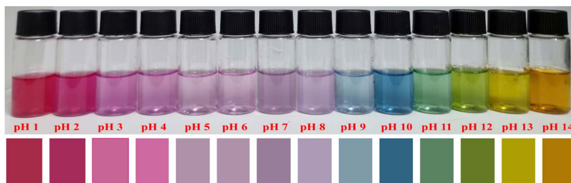
Fig. 9 Color changes of PCE in different pH environments.
