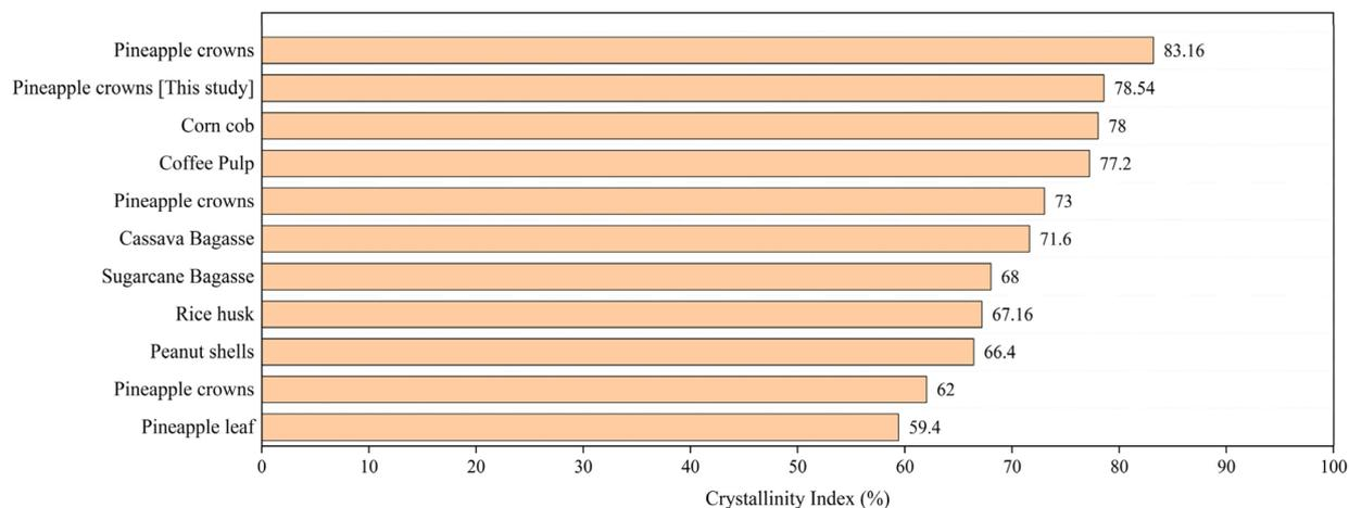
Fig. 6 Crystallinity index of CFs compared across biomass sources.
