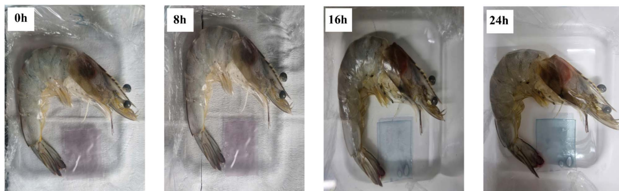
Fig. 10 Color response of bioplastic films containing the anthocyanin extract for real-time monitoring of shrimp freshness at room temperature.
