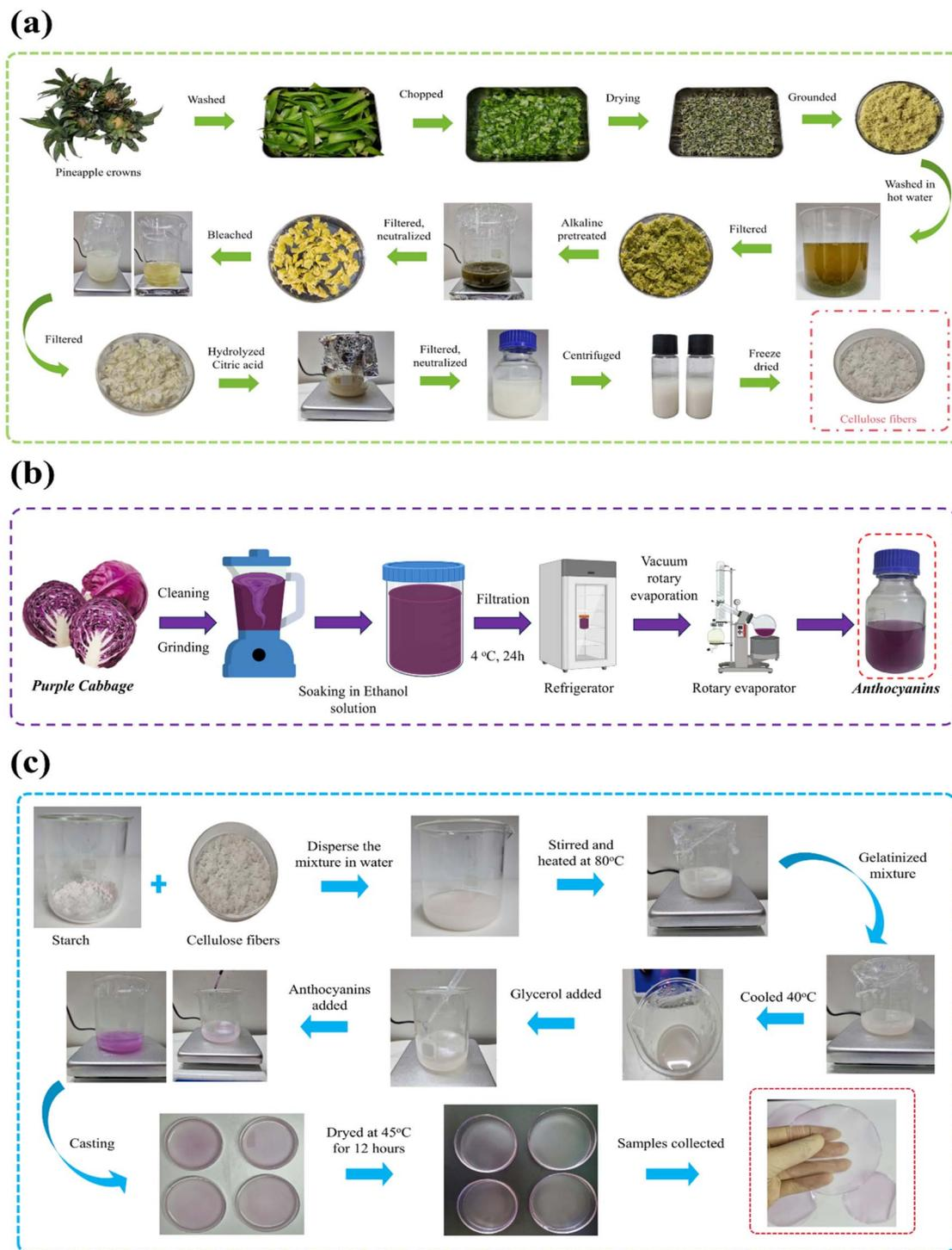
Fig. 1 Cellulose fiber extraction process (a), anthocyanin extraction process (b), and bioplastic film manufacturing process (c).
