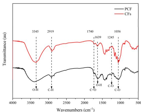
Fig. 4 FTIR spectra of PCF and CFs.
