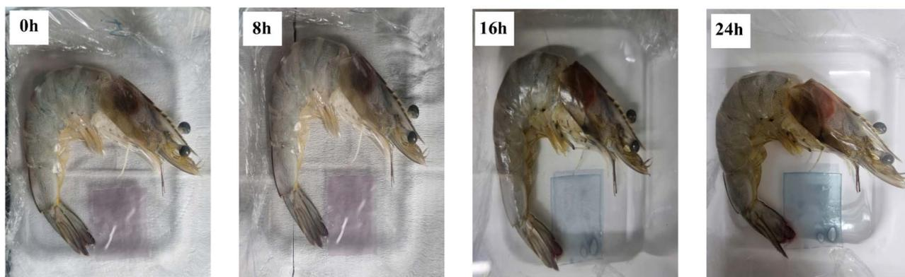
Fig. 10 Color response of bioplastic films containing the anthocyanin extract for real-time monitoring of shrimp freshness at room temperature.
