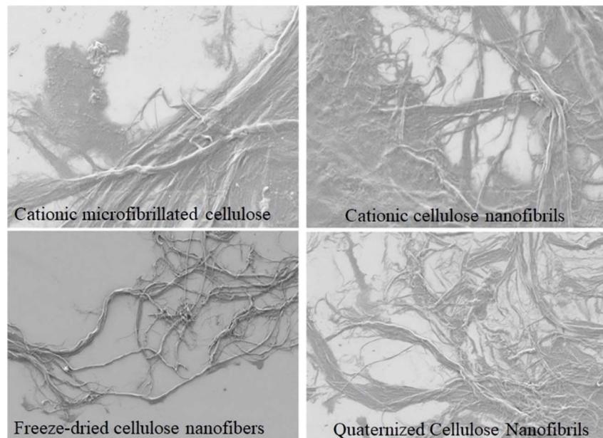
Fig. 10 Micrographs of different types of cellulose-based nanofibers. Published under the CC-BY License.<sup>177</sup> Copyright 2022, The authors. Springer Nature B.V.
