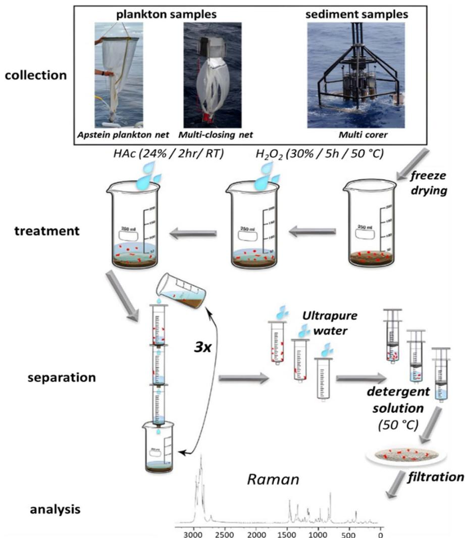
Fig. 6 Workflow for MP detection: (1) sampling via multi-corers or plankton nets; (2) freeze-drying and digestion with H<sub>2</sub>O<sub>2</sub> and acetic acid; (3) separation using syringe cascade and detergent desorption; (4) analysis by Raman spectroscopy. Published under the CC-BY License.<sup>120</sup> Copyright 2021, The authors. Published by Elsevier B.V.
