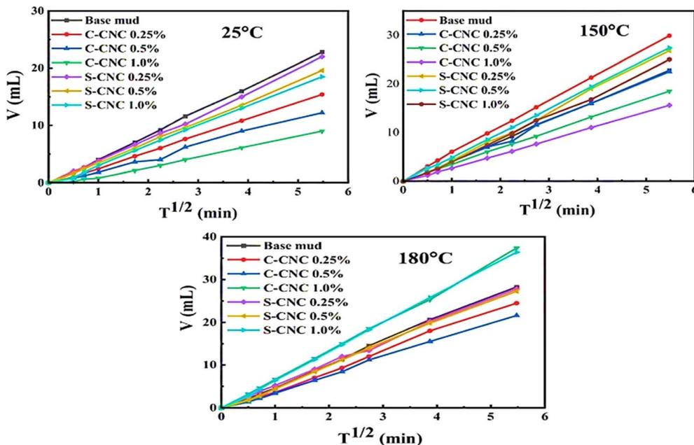
Fig. 9 Filtration volume ( $V$ ) versus square root of time ( $T^{1/2}$ ) for base mud and CNC-modified muds (C-CNC and S-CNC) at 25 °C, 150 °C, and 180 °C, demonstrating the influence of CNC concentration and temperature on fluid loss behavior. Published under the CC-BY License.<sup>170</sup> Copyright 2024, The authors. Published by Springer Nature B.V.
