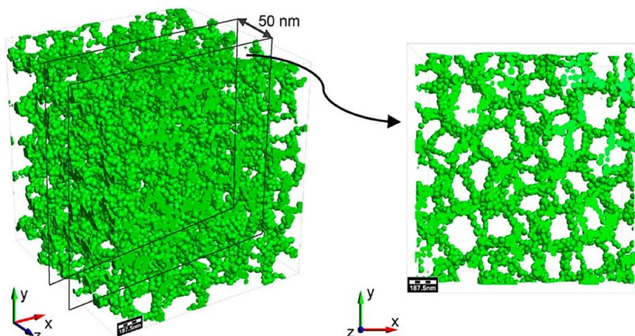
Fig. 20 Aerogel structure comprises atom or nanoparticle clusters forming a solid network (green), with interstitial spaces representing its pores. Published under the CC-BY License.<sup>303</sup> Copyright 2018, The authors. Published by MDPI.
