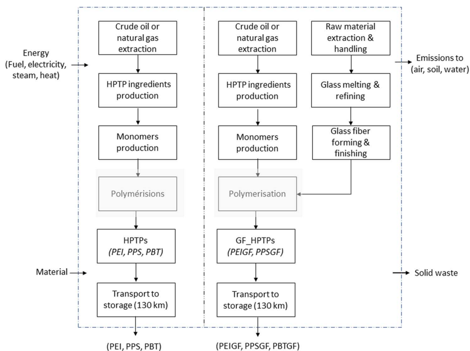
Fig. 1 System boundary of the evaluated HPTP products (PEI = polyetherimide; PEIGF = polyetherimide filled with glass fiber; PPS = polyphenylene sulfide; PPSGF = polyphenylene sulfide filled with glass fiber; PBT = polybutylene terephthalate; PBTGF = polybutylene terephthalate filled with glass fiber).
