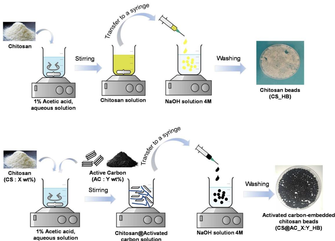
Fig. 1 Multistep preparation of porous chitosan hydrogel beads (CS<sub>HB</sub>) and activated carbon-containing chitosan beads (CS@AC<sub>X:Y</sub><sub>HB</sub>) with X and Y referring to the weight percentage of chitosan and activated carbon, respectively.
