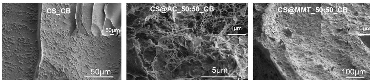
Fig. 3 SEM analysis of CS\_CB, CS@AC\_50:50\_CB and CS@MMT\_50:50\_CB.
