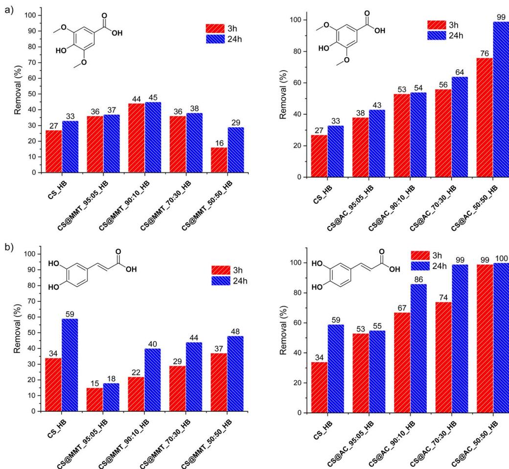
Fig. 5 Effect of the filler loading on (a) the syringic acid uptake and (b) the caffeic acid uptake using chitosan entrapping montmorillonite CS@MMT\_X:Y\_HB and chitosan entrapping activated carbon CS@AC\_X:Y\_HB.
