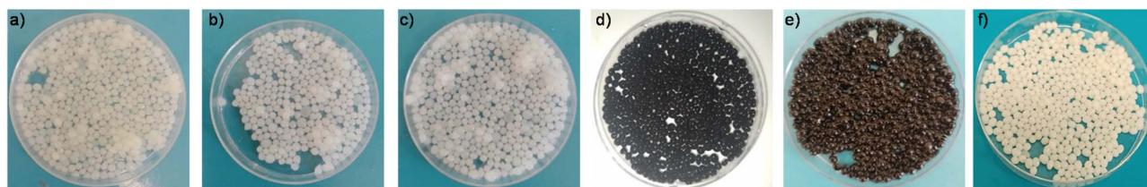
Fig. 2 Chitosan beads entrapping different fillers: (a) CS@MMT<sub>90:10</sub><sub>HB</sub>, (b) CS@HNT<sub>90:10</sub><sub>HB</sub>, (c) CS@SEP<sub>90:10</sub><sub>HB</sub>, (d) CS@AC<sub>90:10</sub><sub>HB</sub>, (e) CS@rGO<sub>90:10</sub><sub>HB</sub>, and (f) CS@C<sub>3</sub>N<sub>4</sub><sub>90:10</sub><sub>HB</sub>.
