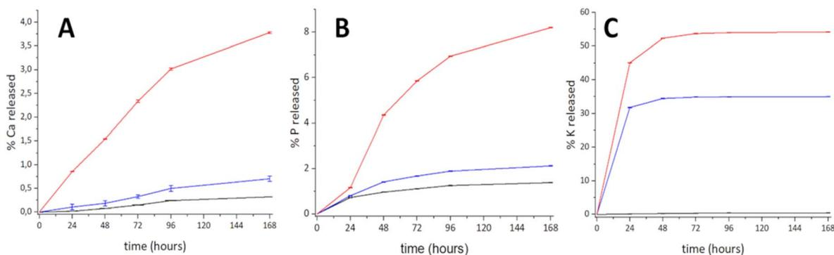
Fig. 4 Cumulative wt% of released Ca (A), P (B) and K ions (C) in water from Hap-1 (black), Hap-2 (blue) and Hap-3 (red).
