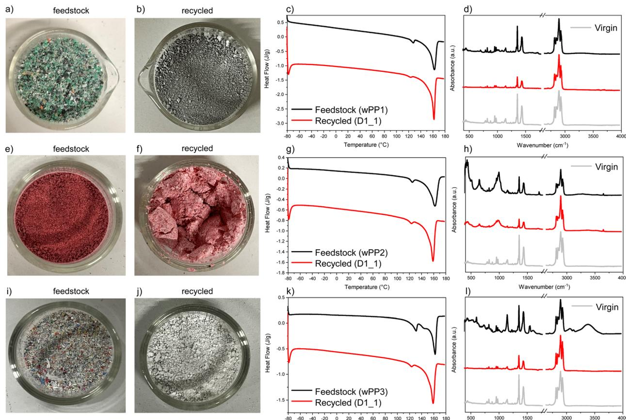
Fig. 7 (a) wPP1, (b) wPP1 recycled in *n*-decane at 130 °C during 30 min, (c) associated DSC heating thermograms, (d) associated IR spectra, (e) wPP2, (f) wPP2 recycled in decane at 130 °C during 30 min, (g) associated DSC heating thermograms, (h) associated IR spectra, (i) wPP3, (j) wPP3 recycled in *n*-decane at 130 °C during 30 min, (k) associated DSC heating thermograms, (l) associated IR spectra.
