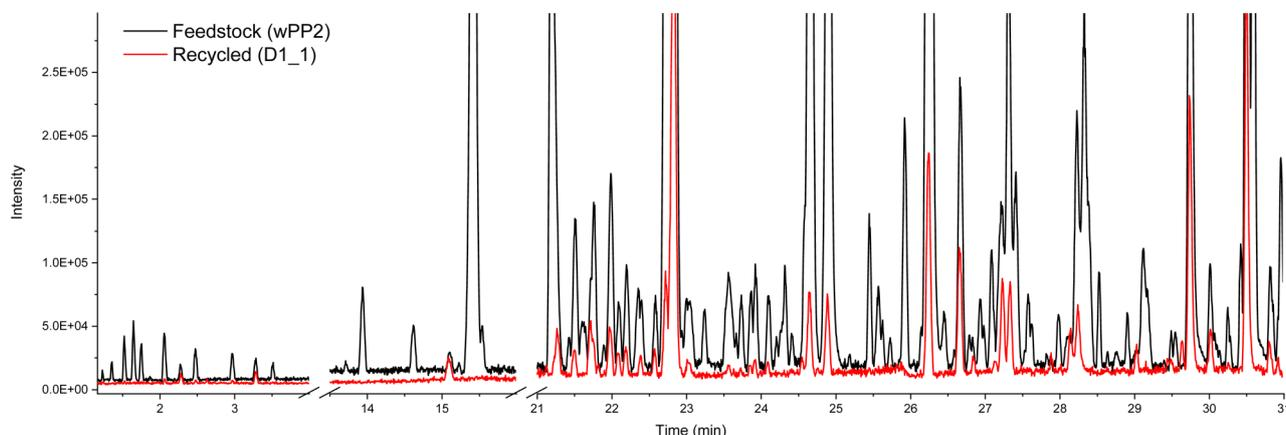
Fig. 8 LC-HRMS chromatogram of the plastic charge wPP2 and the recycled polymer in the D1\_1 operating condition.
