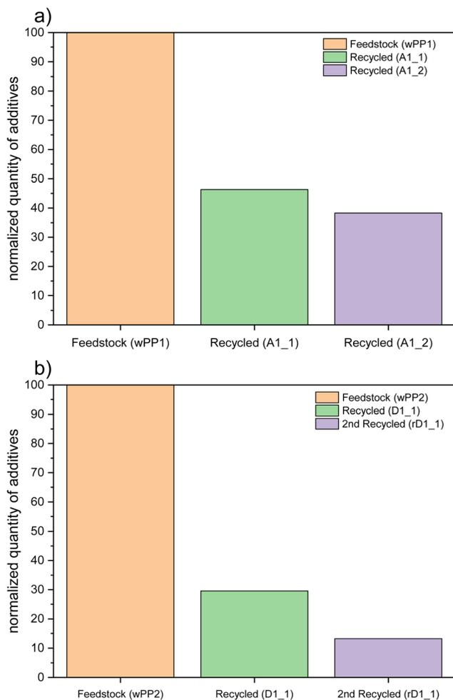
Fig. 9 Normalized quantity of additives obtained from the semi-quantitative approach for wPP1 and the recycled polymer during A1\_1 and A1\_2 operating condition (a) and for wPP2 and the recycled polymer during D1\_1 and rD1\_1 operating condition (b).
