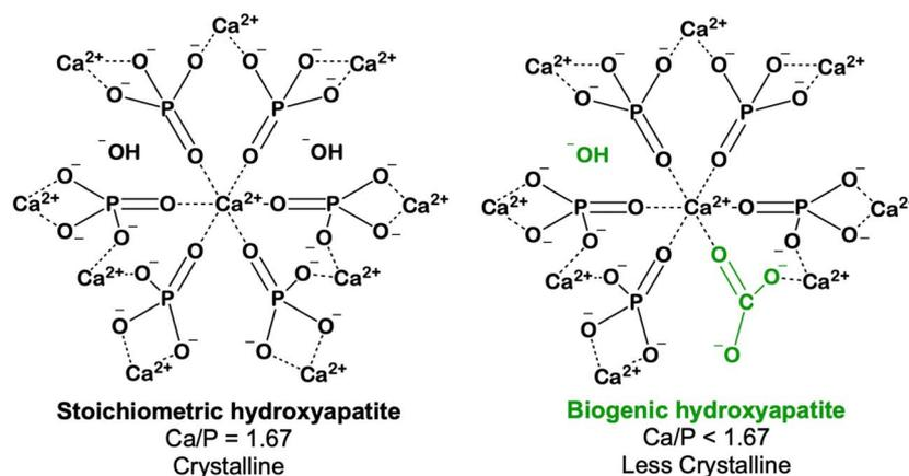
Fig. 4 Structures of stoichiometric HAP,  $\text{Ca}_{10}(\text{PO}_4)_6(\text{OH})_2$  (left) and biogenic HAP,  $\text{Ca}_{10-x}(\text{PO}_4)_{6-x}(\text{CO}_3)_x(\text{OH} \text{ or } \frac{1}{2}\text{CO}_3)_{2-x}$  ( $0 \leq x \leq 2$ ) (right, green).
