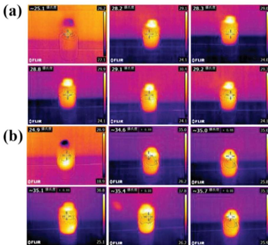
Fig. 12 Changes in temperature for (a) pure water and (b) TS-Co/CoO (0.20). Reproduced with permission from.<sup>70</sup> Copyright (2024), Wiley-VCH Verlag VCH Ltd.
