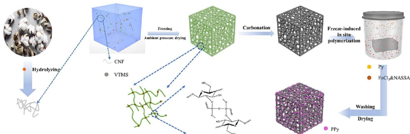
Fig. 2 Schematic of the synthesis of CVCAs-P. Reproduced with permission from.<sup>62</sup> Copyright (2023), Elsevier Inc.
