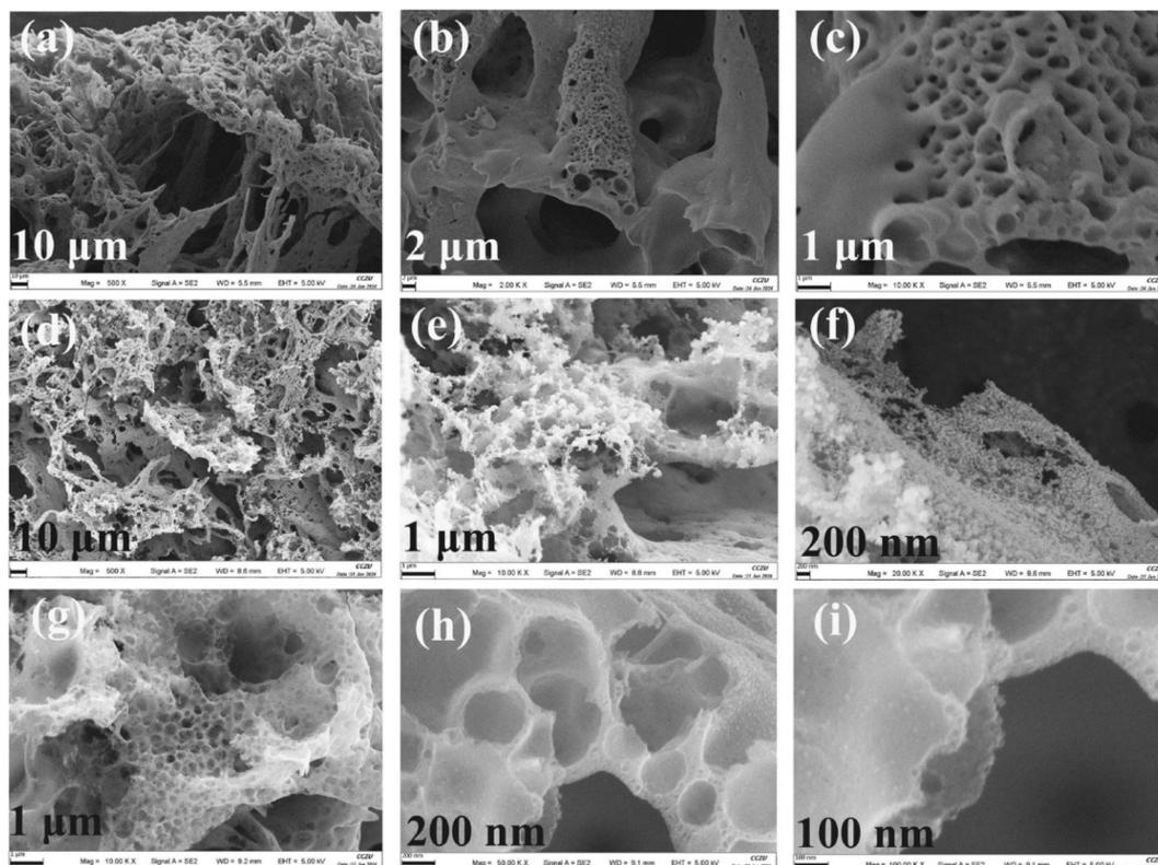
Fig. 9 SEM images of (a–c) AL/APP, (d–f) AL and (g–i) H-AL/APP at different magnifications. Reproduced with permission from.<sup>68</sup> Copyright (2024), Elsevier Inc.
