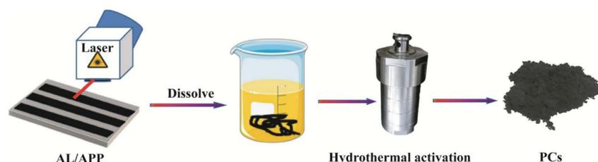
Fig. 8 Pictorial representation for the synthesis of the porous carbon material through LIC and hydrothermal strategies. Reproduced with permission from.<sup>68</sup> Copyright (2024), Elsevier Inc.
