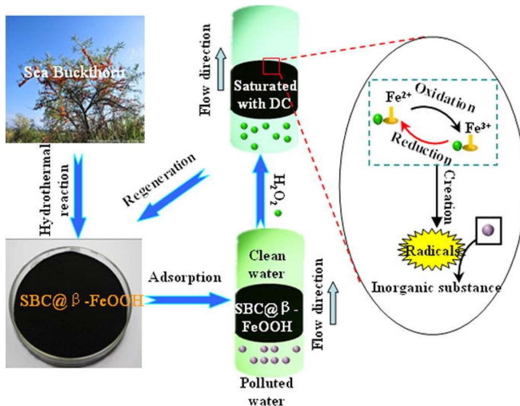
Fig. 7 Schematic of the *in situ* regeneration phenomenon of the SBC@ $\beta$ -FeOOH composite, and its synergistic influence on the removal of aqueous DC solution. Reproduced with permission from.<sup>65</sup> Copyright (2016), Elsevier Inc.
