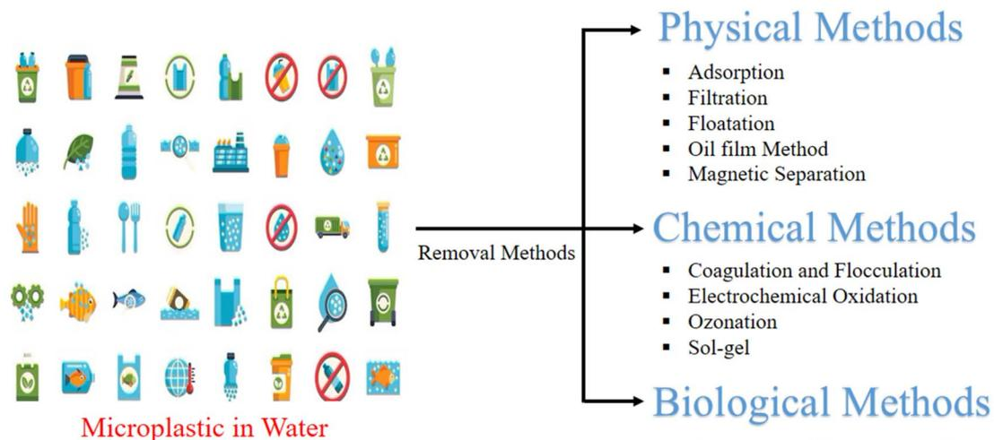
Fig. 8 Overview of the methods used for MP removal from water.
