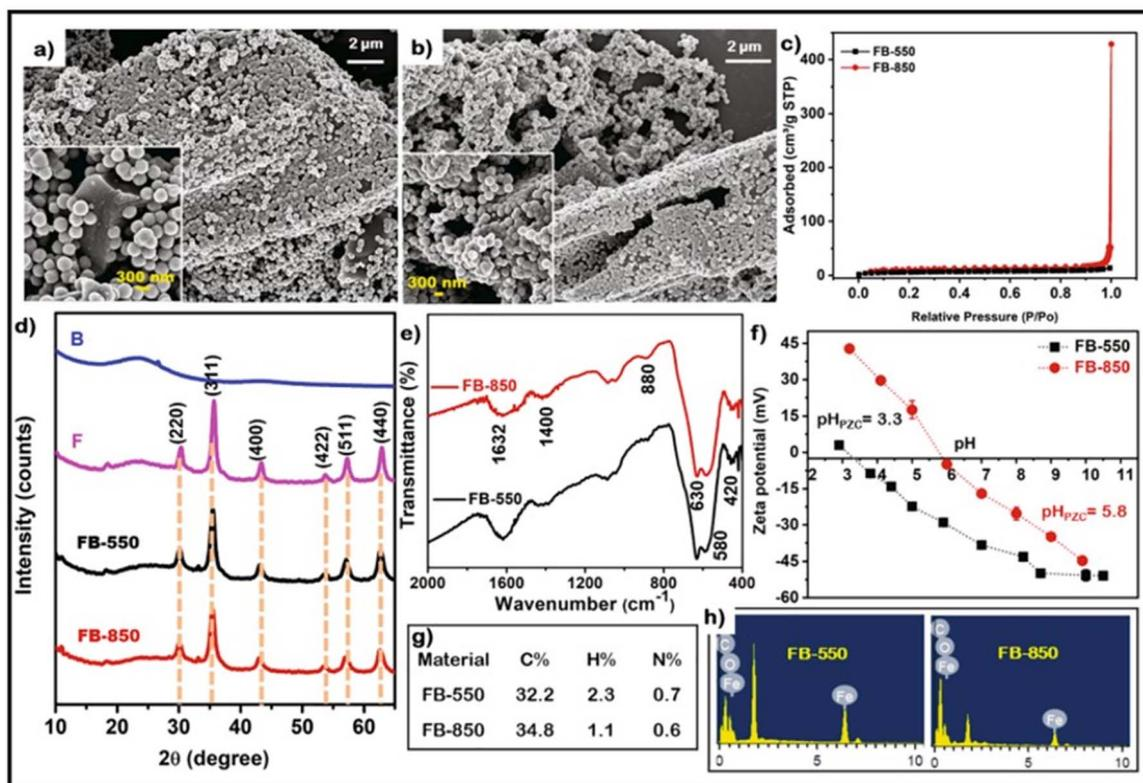
Fig. 7 Iron-modified magnetic biochars (FB), SEM images at (a) 550 °C and (b) 850 °C, (c) gas sorption isotherm for BET analysis, (d) XRD patterns, (e) FTIR spectra, (f) zeta potential vs. pH, (g) CHN elemental analysis, and (h) EDX spectrum. Reproduced with permission from ref. 117, Copyright 2021, Elsevier.
