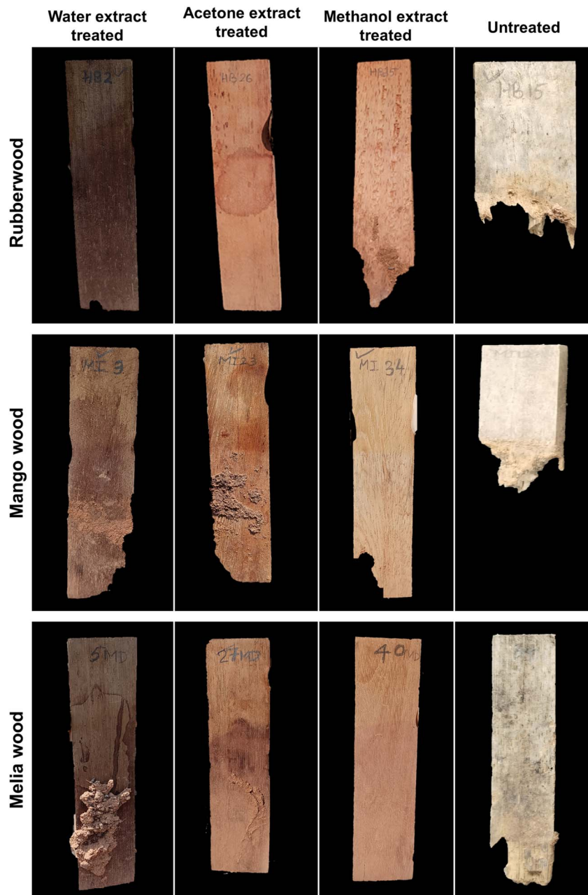
Fig. 2 Degradation against termites in rubberwood, mango wood and melia wood in treated and untreated control wood samples.
