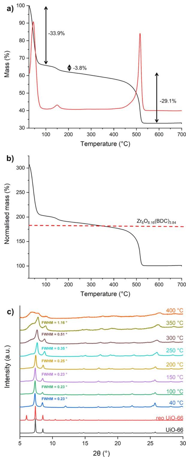
Fig. 5 TG curve of P39 (black) and the respective derivative curve (red) (a); TG curve of P39 with mass normalised to  $ZrO_2$  and the expected normalised mass for the desolvated and dehydroxylated MOF (b); VT-PXRD patterns of P39 from 40 to 400 °C (c).
