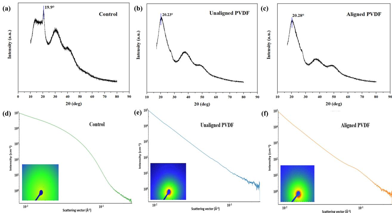
Fig. 3 Comparison of (a–c) XRD spectra for evaluating the crystallinity percentage; (d–f) scattering pattern and plot using SAXS analysis between control ( $\alpha$ -PVDF), unaligned, and aligned PVDF nanofibers.
