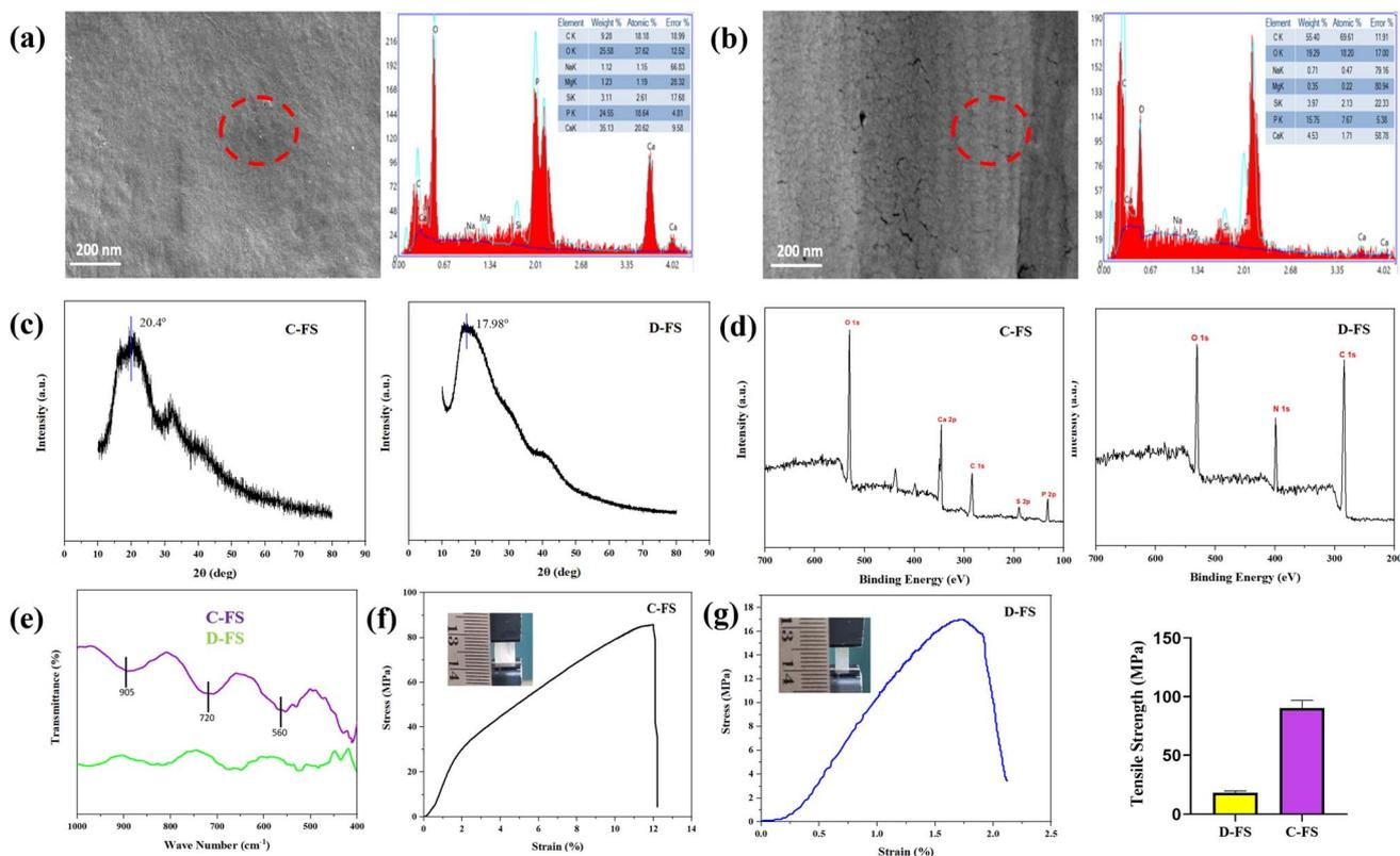
Fig. 5 (a) SEM and EDX analysis of C-FS, with a scale bar of 200 nm; (b) SEM and EDX analysis of D-FS, with a scale bar of 2  $\mu\text{m}$ ; (c) XRD spectra for analysis of crystallinity percentage of C-FS and D-FS; comparison of (d) XPS spectra for elemental analysis; (e) FTIR spectra; (f) decrease in tensile strength due to demineralization of C-FS; (g) stress–strain graphs of C-FS and D-FS.
