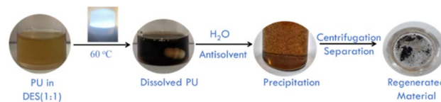
Scheme 1 Pictorial presentation of dissolution of PU in DES (LA : ZnCl 2 = 1 : 1) and its regeneration using water.
