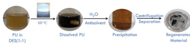
Scheme 1 Pictorial presentation of dissolution of PU in DES (LA : ZnCl<sub>2</sub> = 1 : 1) and its regeneration using water.
