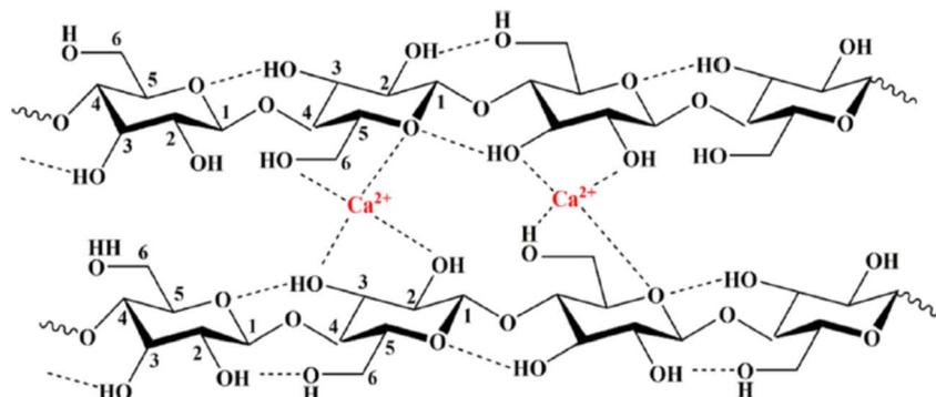
Fig. 5 Interactions of Ca<sup>2+</sup> with cellulose molecules. Reproduced from ref. 103 with permission from the American Chemical Society,<sup>103</sup> copyright 2020.
