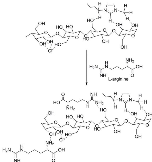
Fig. 6 Cellulose degradation and the mechanism of inhibition of cellulose degradation in  $[C_4mim]Cl$  by L-arginine. Reproduced from ref. 105 with permission from The Royal Society of Chemistry,<sup>105</sup> copyright 2019.
