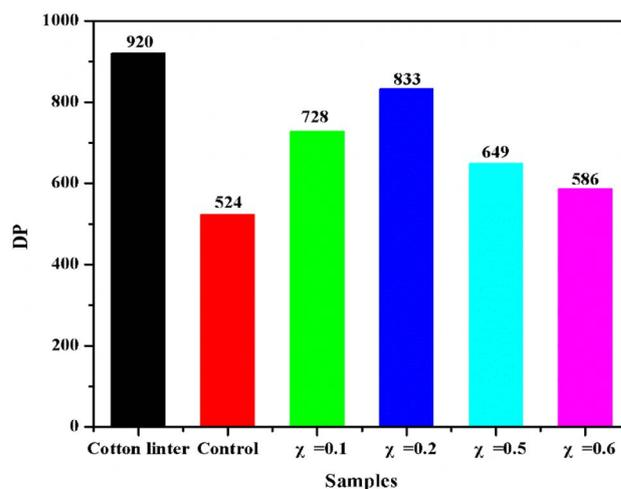
Fig. 4 DP of regenerated cellulose films prepared in mixtures of DMSO/[C<sub>2</sub>mim][OAc] with different IL molar fractions ( $\chi$ ). Reproduced from ref. 101 with permission from Springer Nature,<sup>101</sup> copyright 2017.
