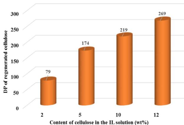
Fig. 3 DP of regenerated cellulose from [N<sub>6222</sub>][OAc] solution as a function of cellulose content (this figure was drawn based on data provided in ref. 95).
