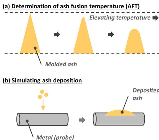
Fig. 4 Typical methods for evaluating ash adhesion at high temperatures. (a) Determining the ash fusion temperature (AFT) and (b) simulating ash deposition.
