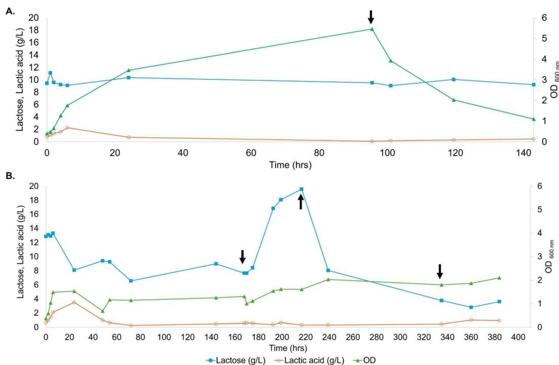
Fig. 5 Continuous fermentation with reduced nutrients. Panel A: aerobic fermentation with airflow set to 0.2 Lpm. Arrow indicates air shut off. Panel B: second attempt at reduced nutrients continuous fermentation with no airflow. From left to right, First arrow = lactose increased to  $20 \text{ g L}^{-1}$ . Second arrow = lactose decreased to  $5 \text{ g L}^{-1}$ . Third arrow = yeast extract increased to  $7.5 \text{ g L}^{-1}$ .
