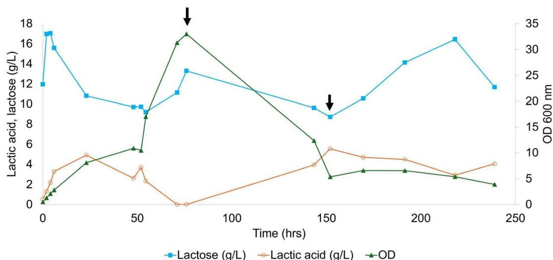
Fig. 4 Continuous fermentation of *L. plantarum* ATCC 8014. Aerobic conditions for growth and lactic acid production were attempted for the first 76 hours after which air supply was turned off (first black arrow, from left to right) due to inhibition of lactic acid production. At 152 hours (second black arrow), lactose was increased from  $15 \text{ g L}^{-1}$  to  $20 \text{ g L}^{-1}$ . See Table 2 for productivity values.
