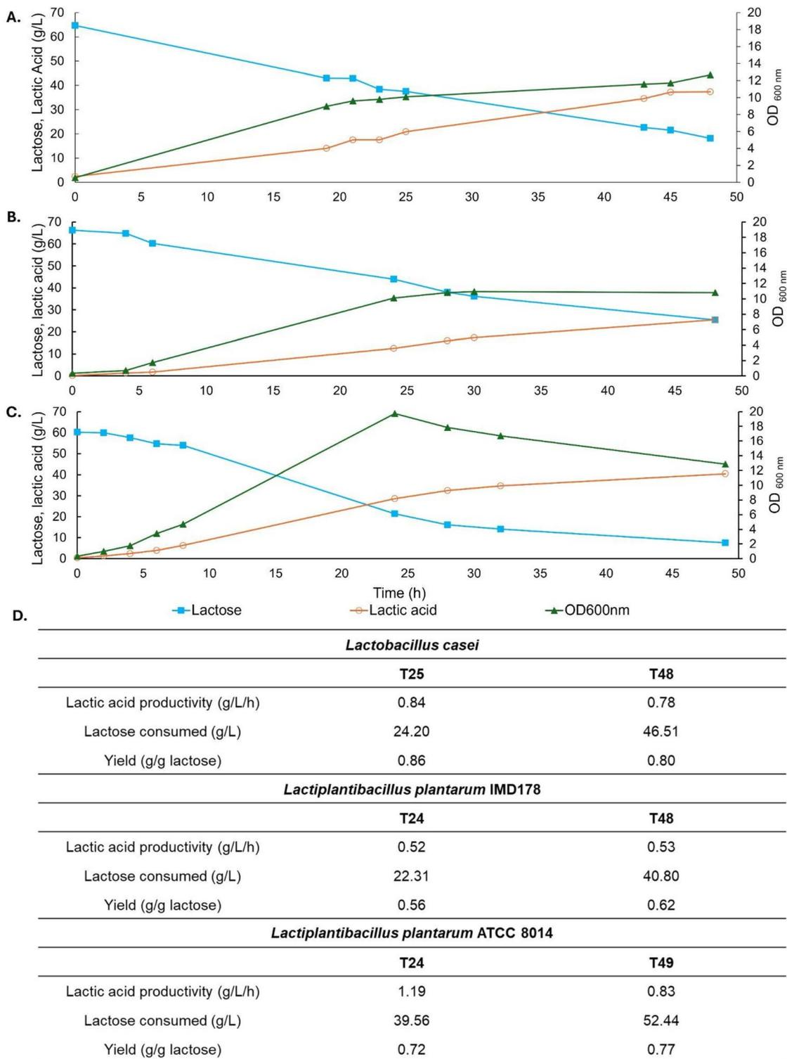
Fig. 1 Batch fermentations under microaerobic conditions in 1 L bioreactors. OD<sub>600nm</sub> measurements were taken via spectrophotometer while lactose and lactic acid measurements were via HPLC. Panel A = *L. casei*, B = *L. plantarum* IMD178, C = *L. plantarum* ATCC 8014, D = table of productivity calculations. Each strain was tested in 1 L bioreactor supplied with  $60 \text{ g L}^{-1}$  lactose, stirring at 200 rpm and no aeration over 48–49 hours.
