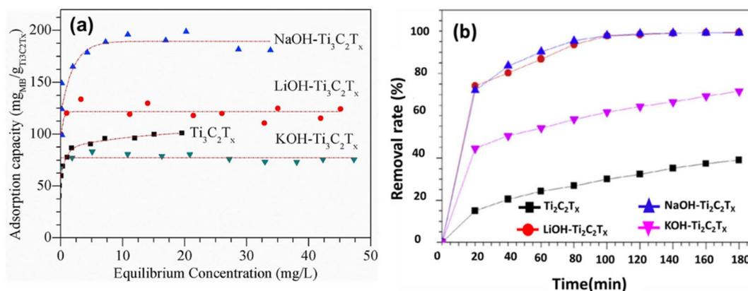
Fig. 8 (a) Plot of the MB removal rate vs. time for different adsorbents. (b) Adsorption isotherms of MB on Ti<sub>3</sub>C<sub>2</sub>T<sub>x</sub>, LiOH-Ti<sub>3</sub>C<sub>2</sub>T<sub>x</sub>, NaOH-Ti<sub>3</sub>C<sub>2</sub>T<sub>x</sub>, and KOH-Ti<sub>3</sub>C<sub>2</sub>T<sub>x</sub>. Reprinted from ref. 116 with permission from Elsevier, *Mater. Chem. Phys.*, Copyright 2018.
