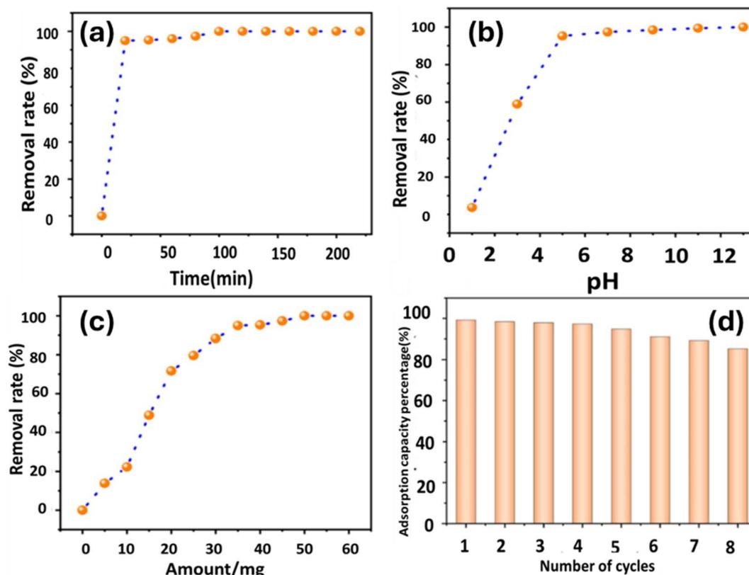
Fig. 5 (a–c) Effect of adsorbent (MXenes-LDH) amount, contact time, and pH on Ni<sup>+</sup> adsorption. (d) Reusability of MXenes-LDH. Reprinted from ref. 87 with permission from Elsevier, *Sep. Purif. Technol.*, Copyright 2020.
