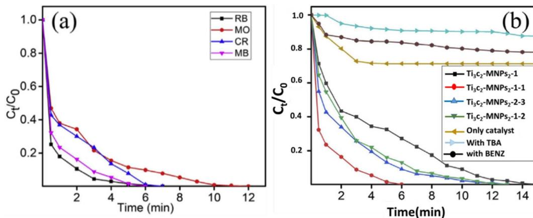
Fig. 9 (a) Degradation efficiencies of  $Ti_3C_2$ -MNPs on four organic dyes. (b) Degradation efficiencies of  $Ti_3C_2$ -MNPs with different mass ratios. Reprinted from ref. 95 with permission from the American Chemical Society, *Environ. Sci. Technol.*, Copyright 2018.
