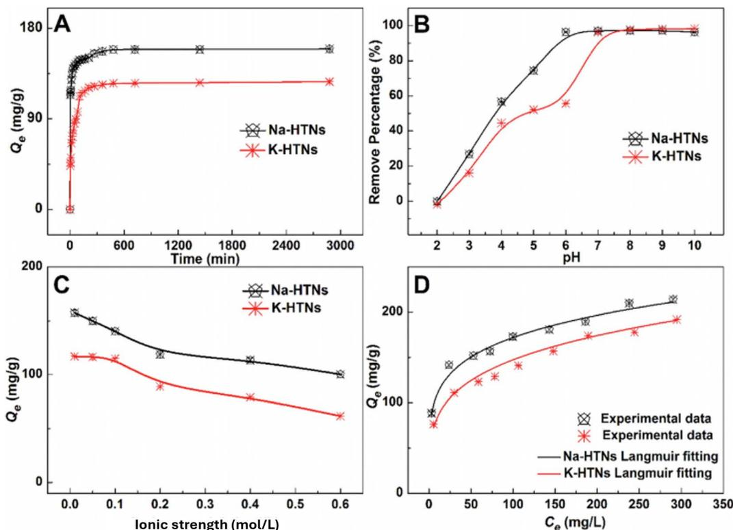
Fig. 7  $\text{Eu}(\text{III})$  removal by MXene-based Na-HTNs and K-HTNs as a function of (A) contact time, (B) pH, (C) ionic strength, and (D) equilibrium concentration. Reprinted from ref. 93 with permission from the Royal Society of Chemistry, *Environ. Sci.: Nano*, Copyright 2020.
