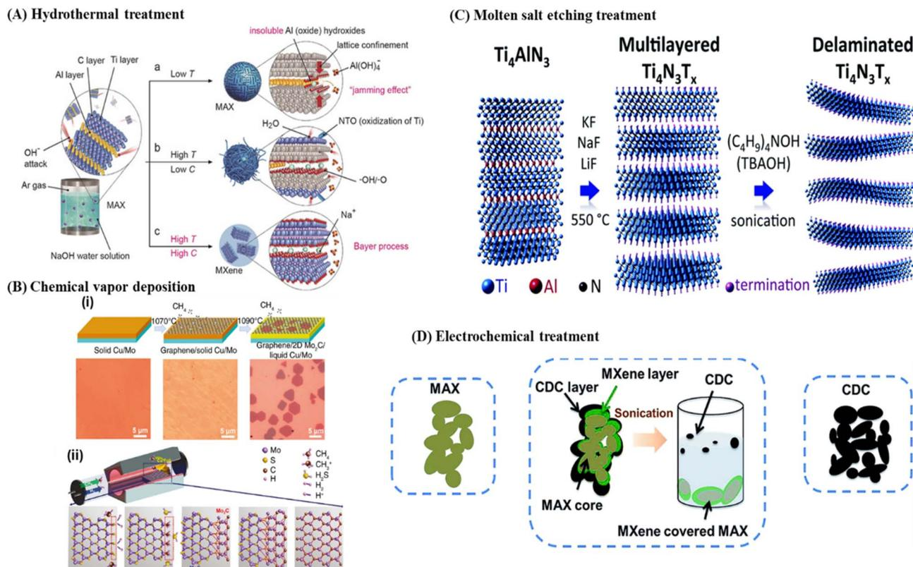
Fig. 4 Schematic of the top-down and bottom-up synthesis approaches for MXenes: (A) hydrothermal treatment, (B) CVD, (C) molten salt etching, and (D) electrochemical treatment. Reprinted from ref. 58 with permission from MDPI, *Molecules*, Copyright 2022.
