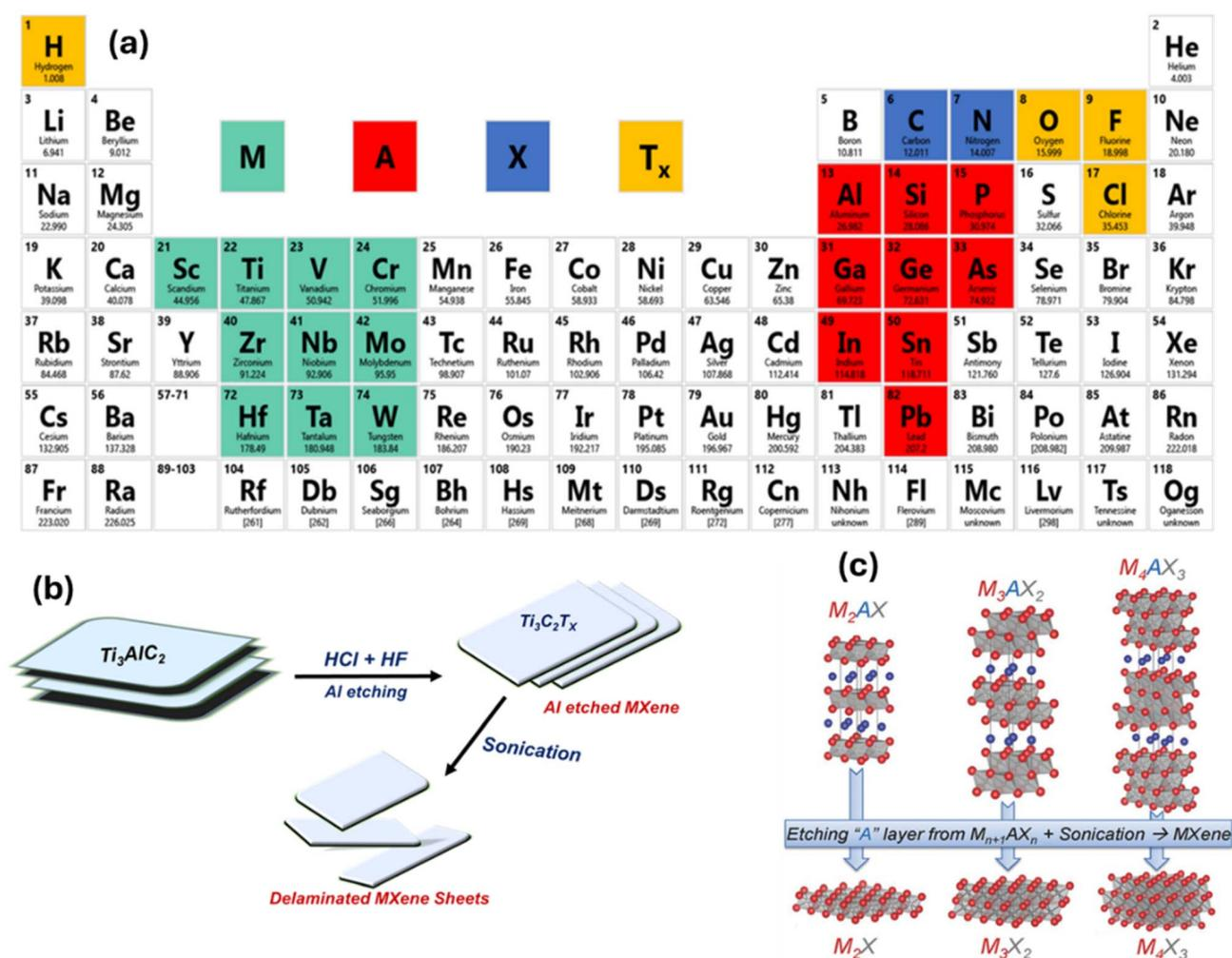
Fig. 1 (a) Elements used in MXene synthesis. Reprinted from ref. 31 with permission from the American Chemical Society, *Chem. Mater.*, Copyright 2018. (b) Schematic of the exfoliation process in the synthesis of  $\text{Ti}_3\text{C}_2\text{T}_x$  MXenes from the max phase. (c) Exfoliation process for  $\text{Ti}_3\text{AlC}_2$ . Reprinted from ref. 53 with permission from Wiley, *Adv. Mater.*, Copyright 2014.
