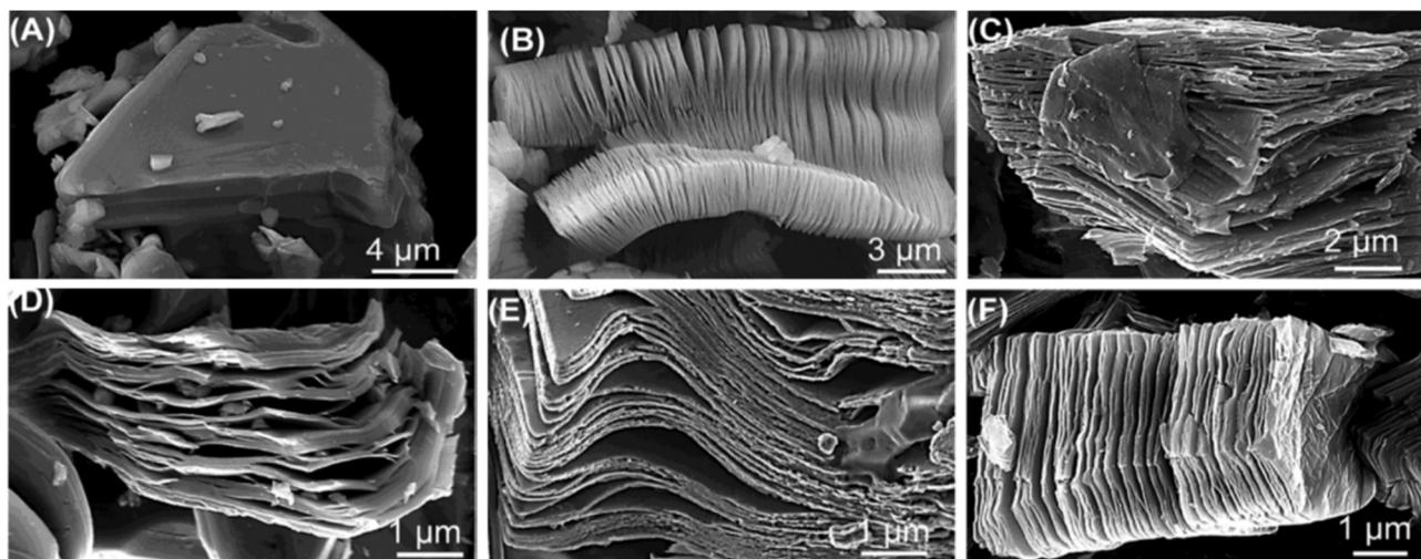
Fig. 3 SEM images for different MXenes: (A) and (B)  $Ti_3AlC_2$  particle before and after ( $Ti_3C_2T_x$ ) HF treatment, (C)  $Ti_2AlC$  after HF treatment, (D)  $Ta_4AlC_3$  after HF treatment, (E)  $TiNbAlC$  after HF treatment, and (F)  $Ti_3AlCN$  after HF treatment. Reprinted from ref. 21 with permission from the American Chemical Society, *Nano*, Copyright 2012.
