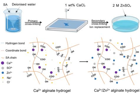
Ca<sup>2+</sup>/Zn<sup>2+</sup> alginate hydrogel electrolyte for high-performance zinc-ion batteries
