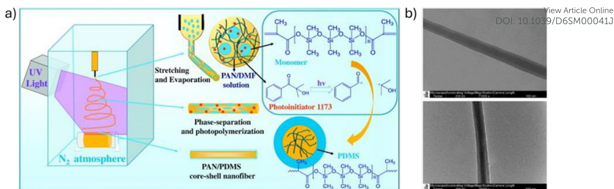
Figure 5. Core-shell fiber architecture generated through phase separation and photopolymerization during electrospinning: (a) schematic representation of the process; (b) TEM images of PAN/PDMS nanofibers prepared at a 2:1 mass ratio. Figure reproduced from Ref 48 with permission from Elsevier B.V., Copyright © 2017.
