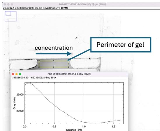
Fig. 4 Quantification of fluorescence intensity of a hydrogel with a tethered concentration gradient of TNF- $\alpha$ . Fluorescence intensity is quantified using the rectangular selection tool and the profile is plotted.
