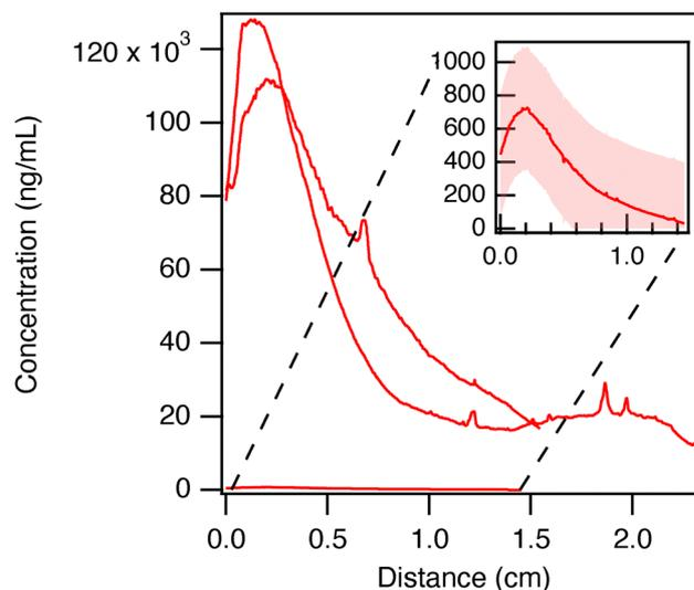
Fig. 9 Individual profiles of hydrogels with tethered TNF- $\alpha$  concentration gradients. The propagation of error from the fit of the calibration curve is shown as the shaded regions behind the solid red lines and is nearly undetectable due to the small error.
