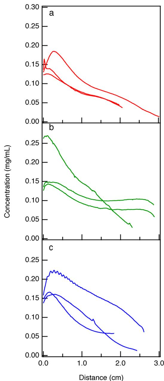
Fig. 7 Individual hydrogel profiles ( $N = 3$ ) with tethered concentration gradients of FITC-PEG-SH after diffusion for (a) 6, (b) 24 or (c) 48 hours. The solid line is the average measured concentration in each device and the shaded region is the propagation of error from the calibration curve fit and is undetectable due to the small error.
