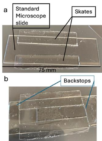
**Fig. 3** Assembly of a device for molecular concentration gradient formation. First (a) symmetric glass rectangles (skates) are cut and glued onto a standard microscope slide and then (b) rectangular backstops are glued at the end of the channels. This is done to create reservoirs for diffusing solutions at either end of the channel and to ensure one directional diffusion across a hydrogel.
