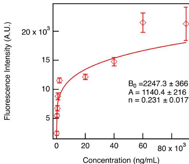
Fig. 8 Calibration curve of measured fluorescence intensity in PEG-N hydrogels with known concentrations of dyed and thiolated TNF- $\alpha$ . Error bars are the standard deviation between measurements ( $N = 5$ ).
