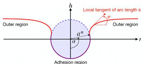
Fig. 2 Schematic of an NPL of radius  $a^*$  wrapped by an initially flat PM. The adhesion region (purple) is described by a contact angle  $\alpha$ , while the outer stretched region (red) is modeled by the tangent angle  $\psi$  along the arclength  $s$ , measured with respect to the horizontal axis  $r$ .
