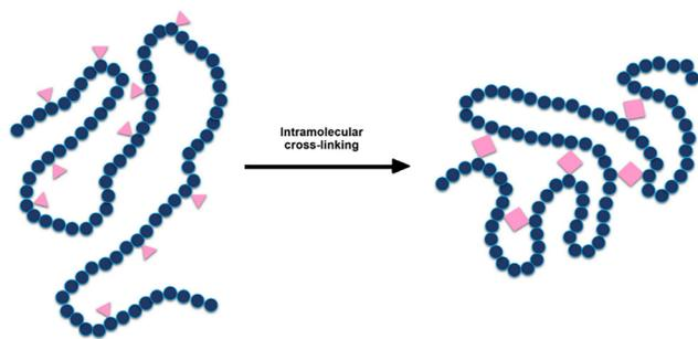
Scheme 1 Representation of intramolecular chain folding, through cross-linking.
