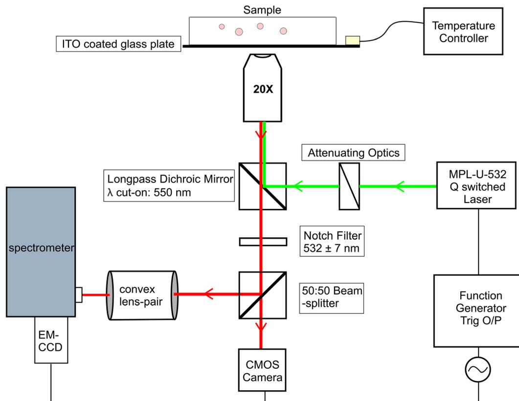
Fig. 2 Schematic picture of the experimental setup.
