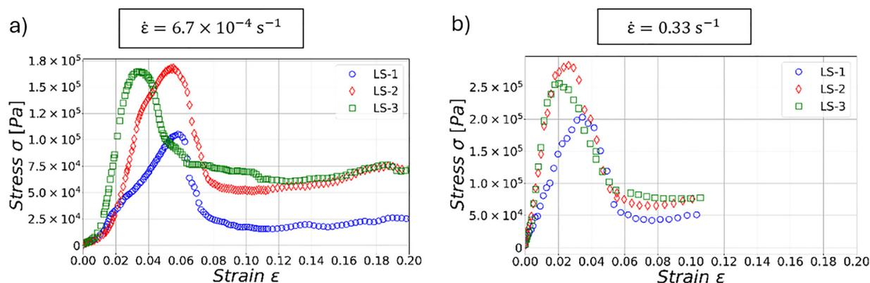
Fig. 14 Stress–strain compression curves of the studied lipsticks LS-1 (blue circles), LS-2 (red diamonds), LS-3 (green squares), obtained at constant displacement rates of  $\dot{\varepsilon} = 6.7 \times 10^{-4} \text{ s}^{-1}$  (a) and  $\dot{\varepsilon} = 0.33 \text{ s}^{-1}$  (b).
