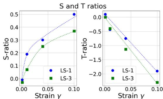
Fig. 11 Evolution of the strain-stiffening ratio ( $S$ -ratio) and shear-thinning ratio ( $T$ -ratio) as a function of strain amplitude during amplitude sweep oscillatory rheological measurements at 1 Hz and 20 °C. Data points for LS-1 are represented by blue circles, and LS-3 by green squares. Dashed lines serve as guidelines.
