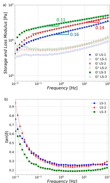
Fig. 8 Frequency sweeps at  $\gamma = 10^{-4}$  of reference lipsticks LS-1 (blue circles), LS-2 (red diamonds), and LS-3 (green squares), representing the evolution of the storage modulus  $G'$  (filled markers) and the loss modulus  $G''$  (empty markers) (a), and the evolution of the loss factor  $\tan(\delta)$  (b), as a function of frequency during oscillatory rheological measurements.
