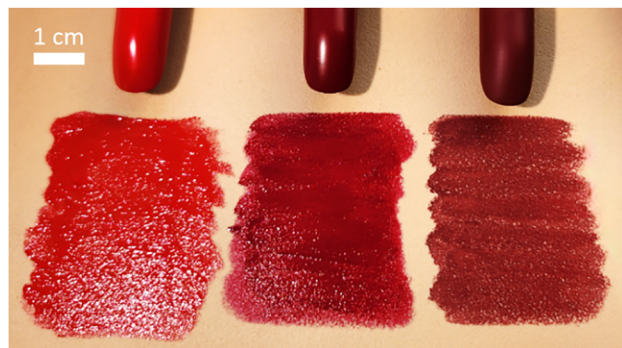
Fig. 1 Lipstick texture rendering after application on synthetic skin of LS-1 (soft and glossy), LS-2 (classic), and LS-3 (hard and matte), from left to right.
