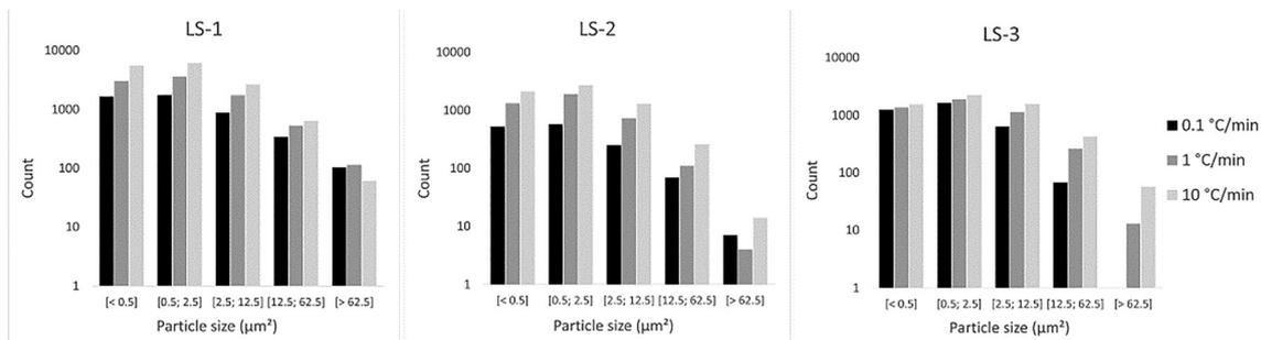
Fig. 4 Particle size distribution histograms (number of particles in each size bin, in log scale) of LS-1, LS-2 and LS-3 measured after cooling at three different rates:  $0.1\text{ °C min}^{-1}$ ,  $1\text{ °C min}^{-1}$  and  $10\text{ °C min}^{-1}$ .
