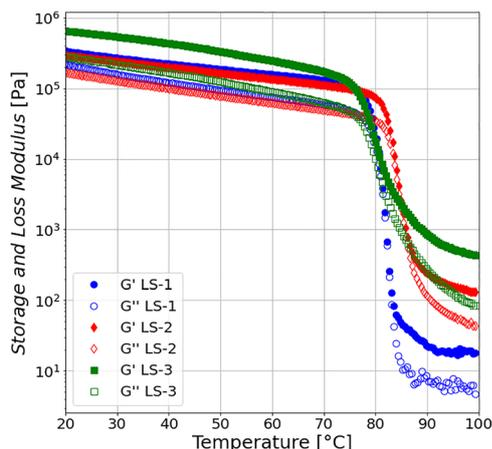
Fig. 6 Thermal sweeps from 100 °C to 20 °C at 1 Hz and  $\gamma = 10^{-4}$  of reference lipsticks LS-1 (blue circles), LS-2 (red diamonds), and LS-3 (green squares), representing the evolution of the storage modulus  $G'$  (filled markers) and the loss modulus  $G''$  (empty markers) as a function of temperature during oscillatory rheological measurements.
