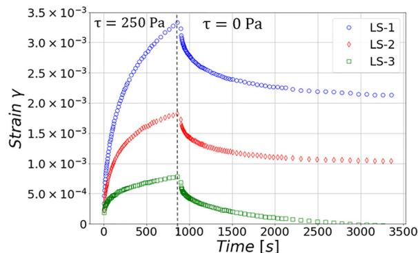
Fig. 12 Overlay of strain curves during shear creep experiments under a torque of 85  $\mu\text{N m}$  corresponding to a mean shear stress of 250 Pa during 900 s and subsequent recovery at 20 °C for LS-1 (blue circles), LS-2 (red diamonds), and LS-3 (green squares).
