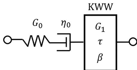
Fig. 2 Schematic representation of the rheological KWW Model.  $G_0$  and  $G_1$  are the shear elastic moduli.  $\eta_0$  is the shear viscosity coefficient.  $\tau$  is the characteristic relaxation time and  $\beta$  is the KWW-exponent.
