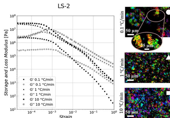
Fig. 5 Rheological oscillatory strain amplitude sweeps at  $20\text{ °C}$  of LS-2 samples subjected to three cooling rates  $0.1\text{ °C min}^{-1}$  (circles),  $1\text{ °C min}^{-1}$  (triangles) and  $10\text{ °C min}^{-1}$  (squares) and corresponding LC-PolScope micrographs.
