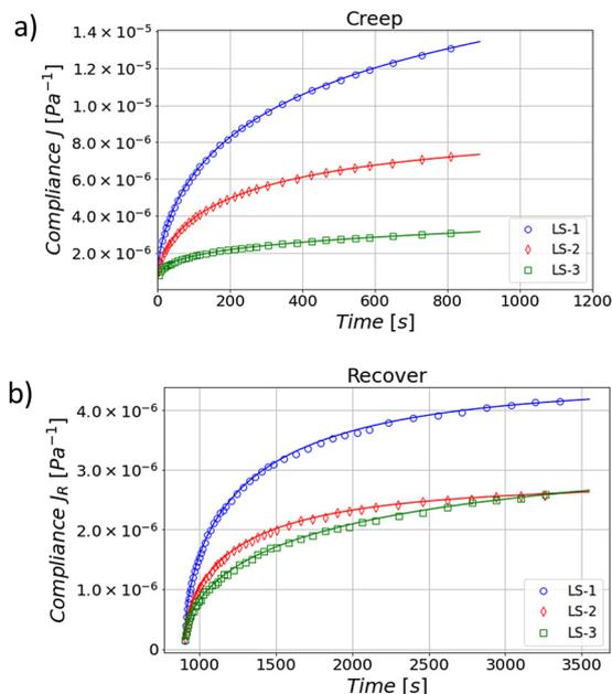
**Fig. 13** Creep compliance curves under 250 Pa (a) and recovery compliance curves (b) with corresponding model determined with the KWW creep model. Experimental data are shown with empty markers, while solid lines represent model predictions.
