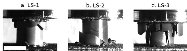
Fig. 15 Post-mortem fracture facies of lipstick samples following uniaxial compression tests shown in Fig. 14a.  $\sim 45^\circ$  cracks are visible for LS-1 (a) and LS-2 (b). Vertical cracks are observed for LS-3 (c). The length of the white scale is 10 mm.
