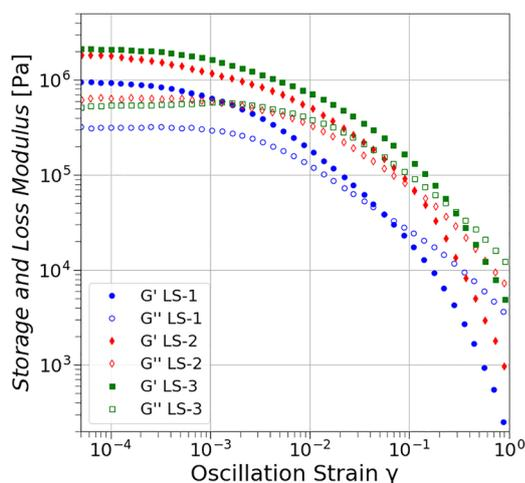
Fig. 7 Strain amplitude sweeps at 1 Hz of reference lipsticks LS-1 (blue circles), LS-2 (red diamonds), and LS-3 (green squares), representing the evolution of the storage modulus  $G'$  (filled markers) and the loss modulus  $G''$  (empty markers) as a function of strain amplitude during oscillatory rheological measurements.
