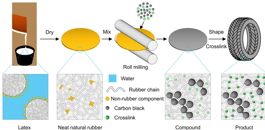
Fig. 5 A conventional method to make a product of carbon black reinforced natural rubber involves several steps, which change the molecular architecture of rubber chains.
