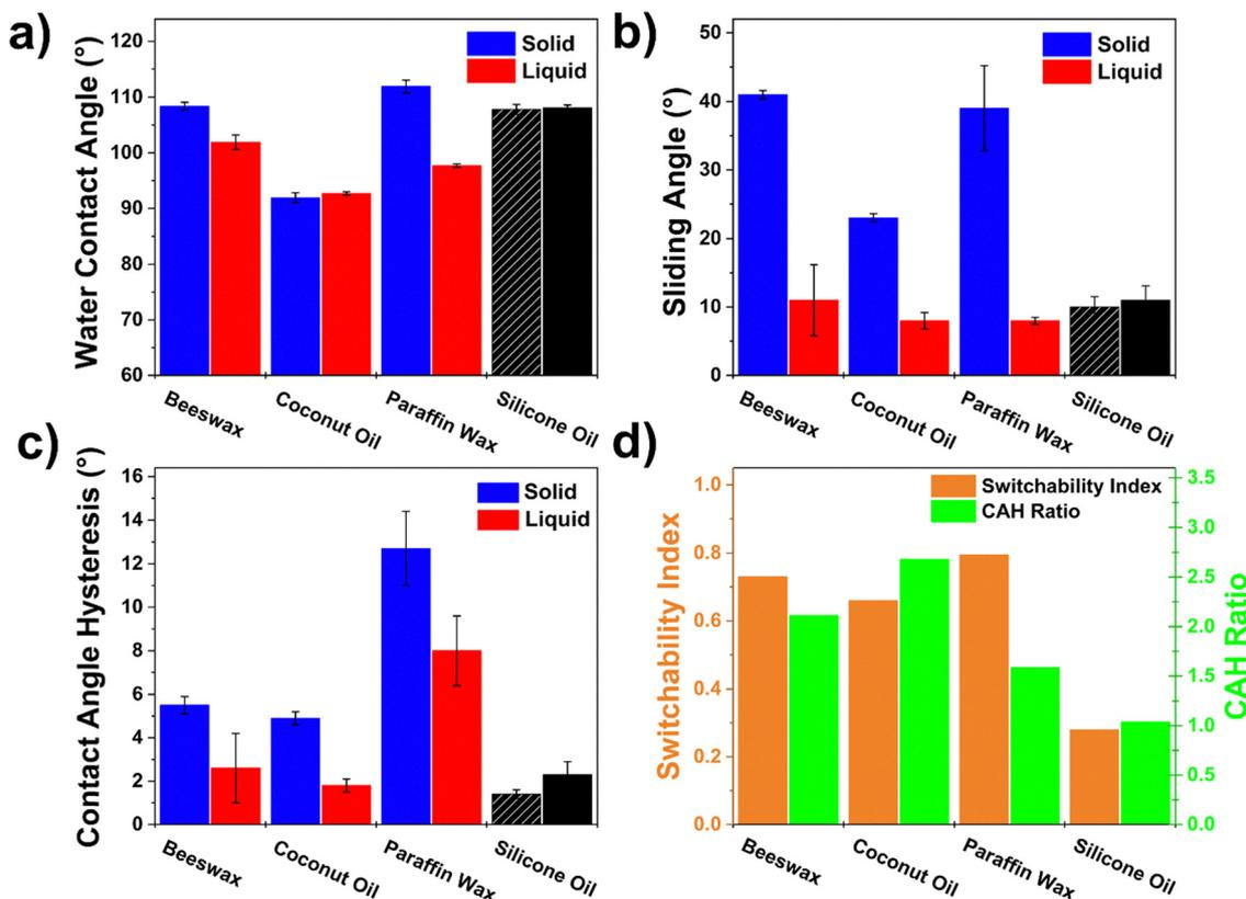
Fig. 2 Wettability of PC-LIS. (a) Static water contact angle (WCA), (b) sliding angle, and (c) contact angle hysteresis (CAH) measurements comparing the solid and liquid phases of each oil, and at two different temperatures for silicone oil (20 °C and 75 °C). (d) Quantification of the switchability index and CAH ratio. For the control, silicone oil, the striped black bar indicates 20 °C and the solid black bar indicates 75 °C.
