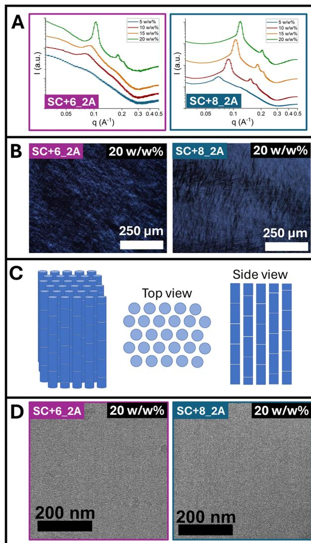
Fig. 1 (A) Small-angle X-ray scattering (SAXS) profiles of SC+6\_2A (left) and SC+8\_2A (right) at 5, 10, 15, and 20 w/w% in Milli-Q water. (B) Polarized optical microscopy (POM) images showing birefringence in SC+6\_2A (left) and SC+8\_2A (right) at 20 w/w% in Milli-Q water. (C) Schematic model for bundlemer packing in hexagonal columnar liquid crystals. (D) Cryo-TEM of SC+6\_2A (left) and SC+8\_2A (right) liquid crystals at 20 w/w% in Milli-Q water.
