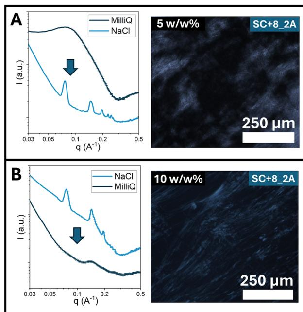
Fig. 6 (A) Order-to-order of SC+8\_2A prepared at 5 w/w% in Milli-Q water, forming nematic liquid crystals confirmed by SAXS (left) and POM (right). After salt addition and sonication, lattice particle formation was confirmed by SAXS (left). (B) Order-to-order transition of SC+8\_2A prepared at 10 w/w% in 0.5 M NaCl, forming lattice particles confirmed by SAXS (left). Following solvent exchange to remove salt, nematic liquid crystal formation was confirmed by SAXS (left) and POM (right).
