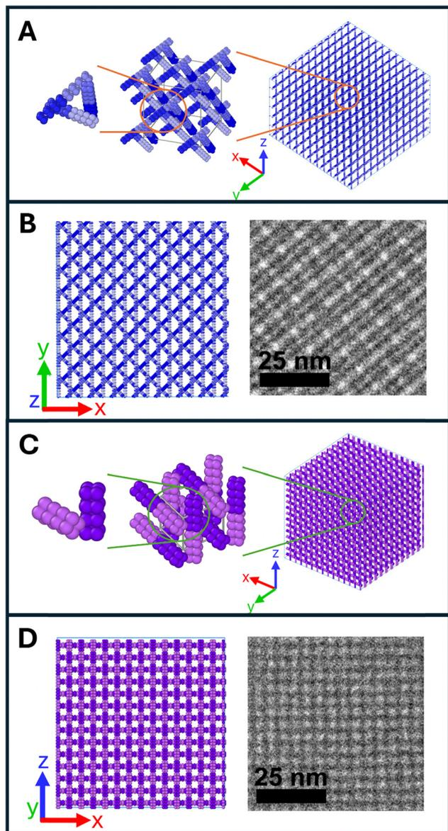
Fig. 4 (A) Lattice packing model of SC+8\_2A derived from experimental SAXS data (Fig. S-19). (B) Projection of the SC+8\_2A lattice SAXS model matched to cryo-TEM images, with different hues highlighting individual bundlemers (applied to both SC+6\_2A and SC+8\_2A). (C) Lattice packing model of SC+6\_2A derived from experimental SAXS data (Fig. S-20). (D) Projection of the SC+6\_2A lattice model matched to cryo-TEM images.
