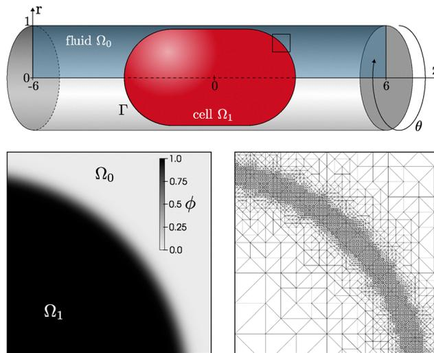
Fig. 1 Simulation setup of a cell in a cylindrical channel. Top: Sharp-interface model with cell ( $\Omega_1$ ) and fluid ( $\Omega_0$ ) separated by interface  $\Gamma$ . Due to axisymmetry, only the blue rectangle is computed. Bottom: Diffuse-interface representation of the inset region by a phase field  $\phi$  (left) and the corresponding adaptive mesh (right).
