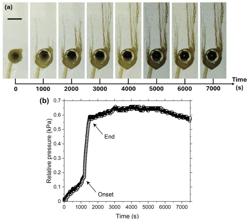
Fig. 2 Results for a representative experiment performed with a  $\text{MgCl}_2$  pellet in a 1.2 M  $\text{Na}_2\text{SiO}_3$  solution. (a) Photographs of the experiment taken every 1000 s, where gravity was operating downwards. The scale bar is 1 cm long. (b) Plot of the relative pressure at the centre throughout the experiment. A sharp increase can be observed at approximately 1200 s whose points of onset and end are marked by arrows.
