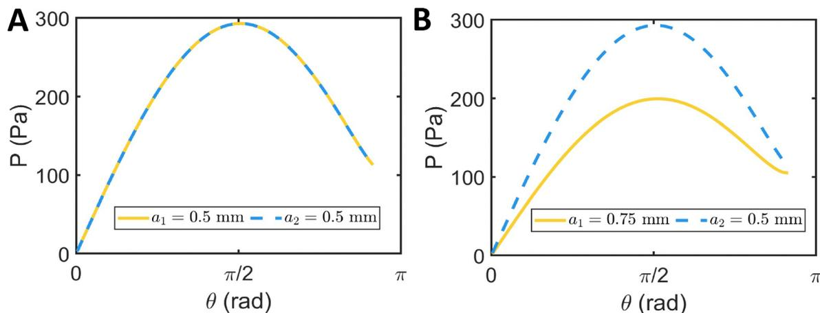
Fig. 4 Droplet pressure. Numerical values of the pressure calculated from eqn (11) as a function of contact angle for individual sessile droplets of (A) equal contact radii,  $a_1 = a_2 = 0.5$  mm, and (B) unequal contact radii,  $a_1 = 0.75$  mm  $a_2 = 0.5$  mm. In all cases, the relation is non-monotonic with a local maximum for  $\theta \approx \pi/2$ . (In the absence of gravity, the maximum pressure occurs for  $\theta = \pi/2$ .)
