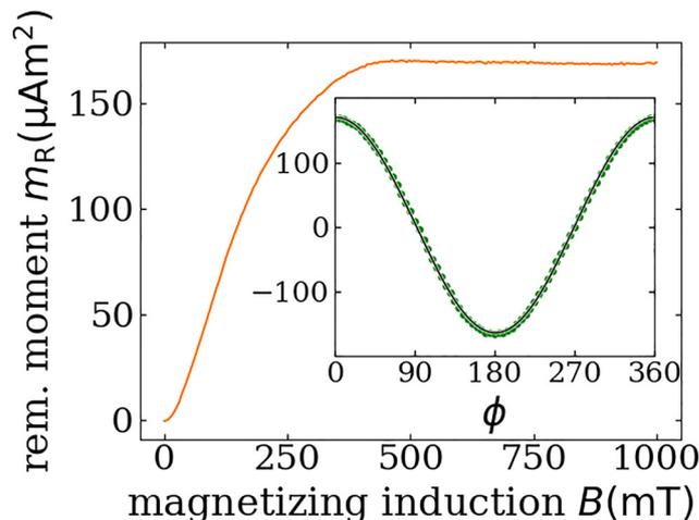
Fig. 5 The isothermal remanent magnetisation curve (IRM) of the utilized steel spheres. The inset displays the measured angular dependence of  $m_{\text{R}}$  magnetized with 1000 mT. The data are marked by green circles. The black line gives a fit by  $m_0 \cos(\phi + \phi_0) + m_1$ , with  $m_0 = 167.1 \mu\text{A m}^2$ ,  $m_1 = 2.7 \mu\text{A m}^2$ , and  $\phi_0 = -1.27^\circ$ .
