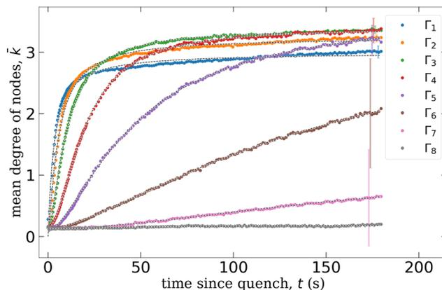
**Fig. 11** Temporal evolution of the mean degree of the nodes for different applied shaking amplitudes, as listed in Table 2 (Section A). To not overload the graphs, for  $t < 4$  s every 5th data point has been plotted, and for  $t > 4$  s only every 15th data point has been plotted. The dashed lines mark fits by eqn (5). All data points and representative error bars have been estimated from 15 independent measurements.<sup>53</sup>
