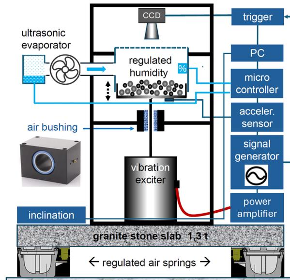
Fig. 2 A sketch of the experimental setup (not to scale). For details of the devices see text.
