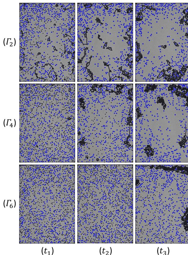
Fig. 6 Emerging structures for a quench from  $\Gamma_{\text{gas}} = 3.3$  g down to increasing shaker amplitudes,  $\Gamma_2 = 1.57$  g,  $\Gamma_4 = 1.73$  g, and  $\Gamma_6 = 1.88$  g. We display the structures for three exemplary times, namely  $t_1 = 5$  s,  $t_2 = 30$  s, and  $t_3 = 150$  s. See also the related movies, 1.57g.mp4, 1.73g.mp4 and 1.88g.mp4, which can be accessed under "files" at <https://doi.org/10.17605/OSF.IO/6S4FM>.
