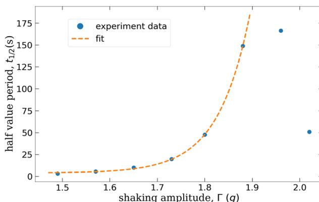
**Fig. 12** Half-value period versus shaking amplitude. The dashed line indicates a fit by eqn (6), where only the data [ $\Gamma_1, \Gamma_6$ ] are taken into account. Fitting parameters are  $t_1 = (1.06 \times 10^{-10} \pm 6.6 \times 10^{-11})$  s,  $\Gamma_c = (6.7 \times 10^{-2} \pm 1.5 \times 10^{-3})$  g and the offset  $t_2 = (4.02 \pm 6.7 \times 10^{-1})$  s.
