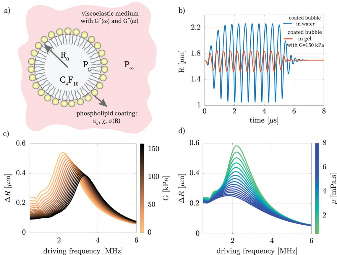
**Fig. 1** (a) Schematic and relevant parameters for a phospholipid-coated microbubble in a viscoelastic medium. (b) Radial response for a coated bubble in water ( $\mu = 1$  mPa s) and in a viscoelastic medium ( $G = 150$  kPa and  $\mu = 1$  mPa s). (c) Resonance curves of a coated microbubble in media with a viscosity of  $\mu = 1$  mPa s and  $G$  ranging from 0 to 150 kPa. (d) Resonance curves of a coated microbubble for media with  $G = 0$  Pa and  $\mu$  ranging from 1 to 8 mPa s.
