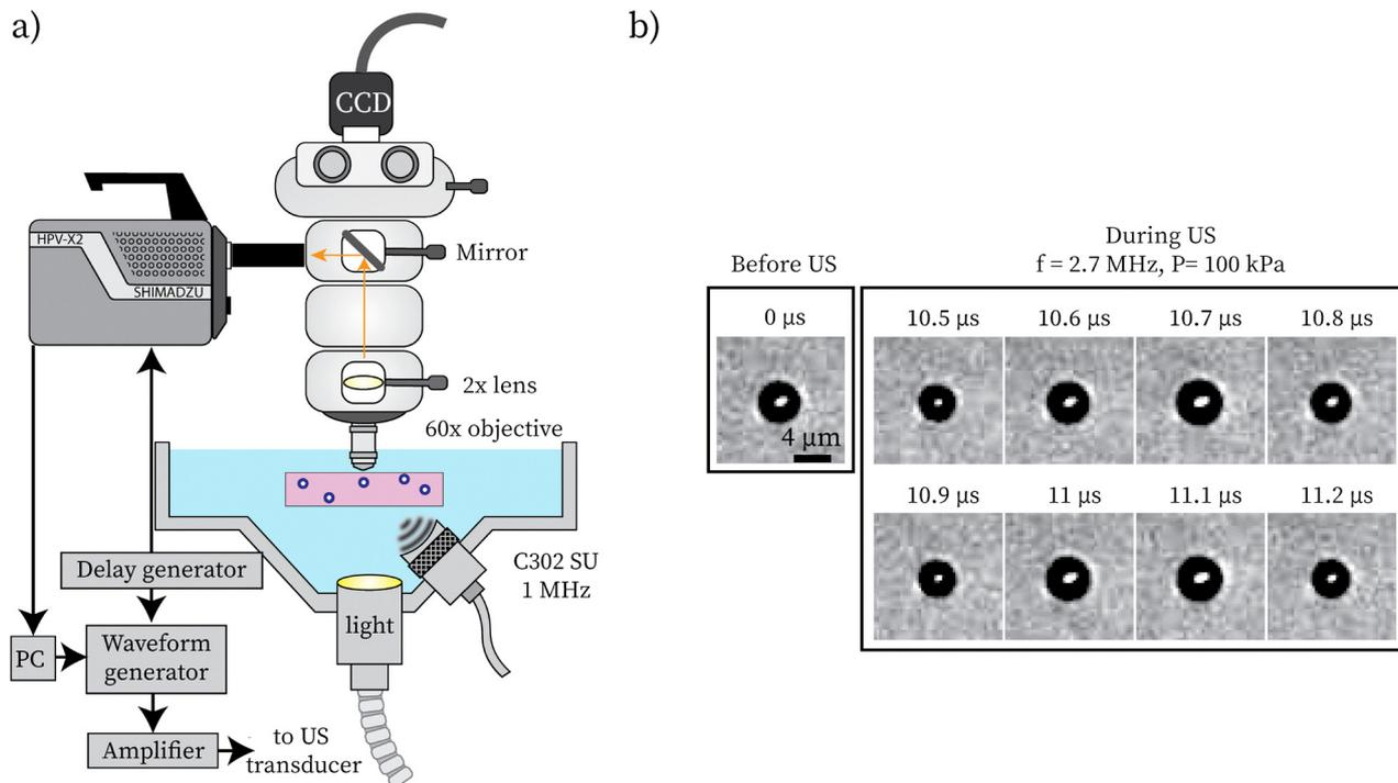
Fig. 2 (a) Schematic of the experimental setup. (b) Snapshots of an ultra-high-speed recording of an oscillating microbubble with an initial radius of  $R_0 = 1.7 \mu\text{m}$  in a soft hydrogel with a shear modulus of  $G(\omega \rightarrow 0) \approx 70 \text{ kPa}$ . The interframe time is 100 ns.
