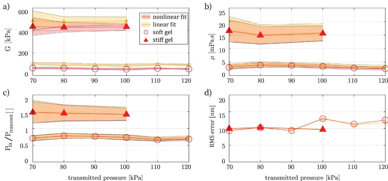
**Fig. 5** (a) Fitted values of  $G$  for the soft and stiff hydrogels, and for the linear and nonlinear fits. (b) Viscosity as a function of the driving pressure. (c) Ratio of the fitted acoustic pressure to the expected acoustics pressure based on the transducer calibration performed in water. (d) Root mean square error in nanometers corresponding to the best linear and nonlinear fits. The error bars (and shadowed region) represent 95% confidence interval on the fitted parameters.
